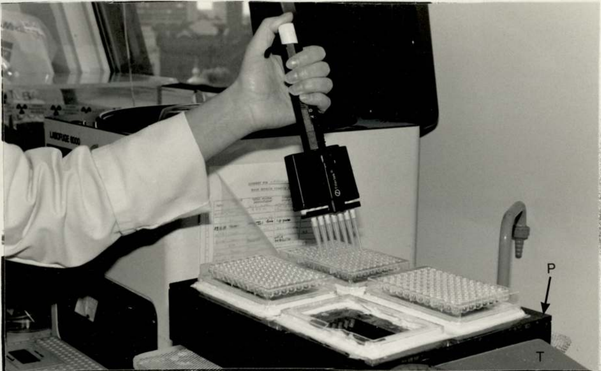
Figure 3. Apparatus for the assay of PKC activity using microtitre plates. A thermostirrer (T) was used to heat and circulate water through the base of 96 well U-form microtitre plates taped securely to the top of a perspex box (P), such that solutions in the microtitre wells were maintained at 32°C.
