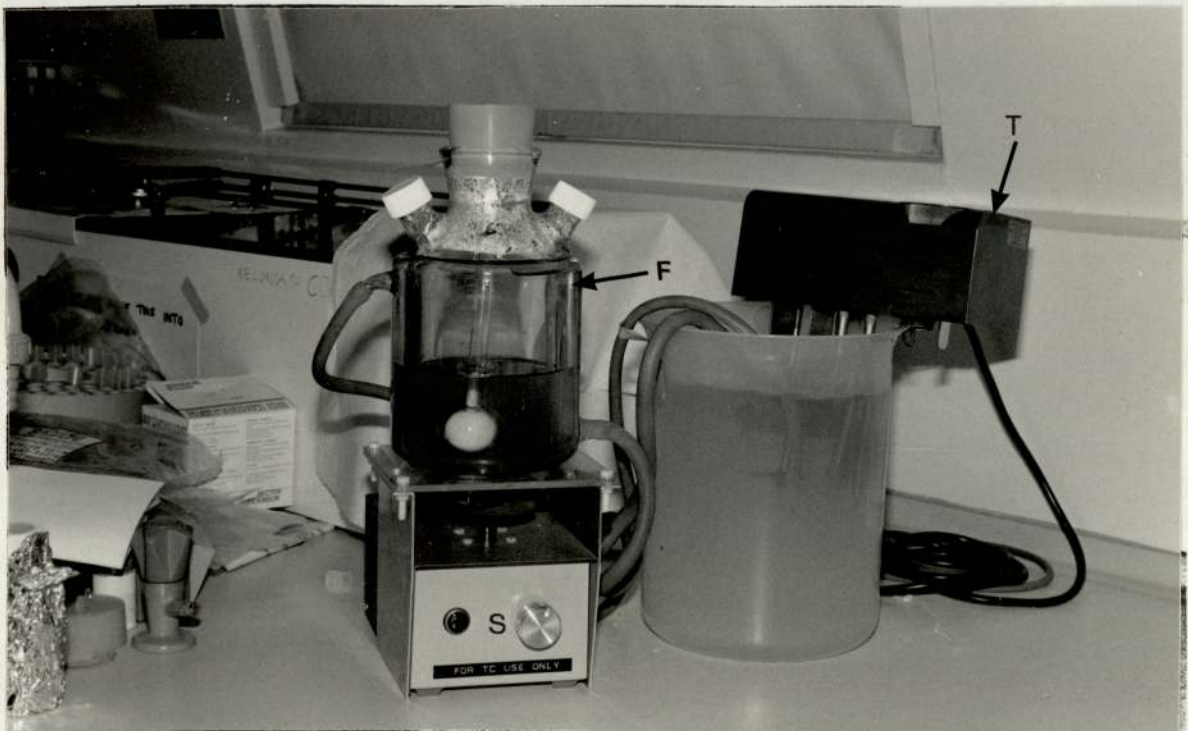
Figure 4. Apparatus for the culture of cells on Cytodex 1 microcarrier beads. Cells were cultured in a silanized culture flask (F) and stirred using a slow speed stirrer (S). Cultures were maintained at 37°C by the circulation of water through a water jacket surrounding the flask using a thermostirrer (T).
