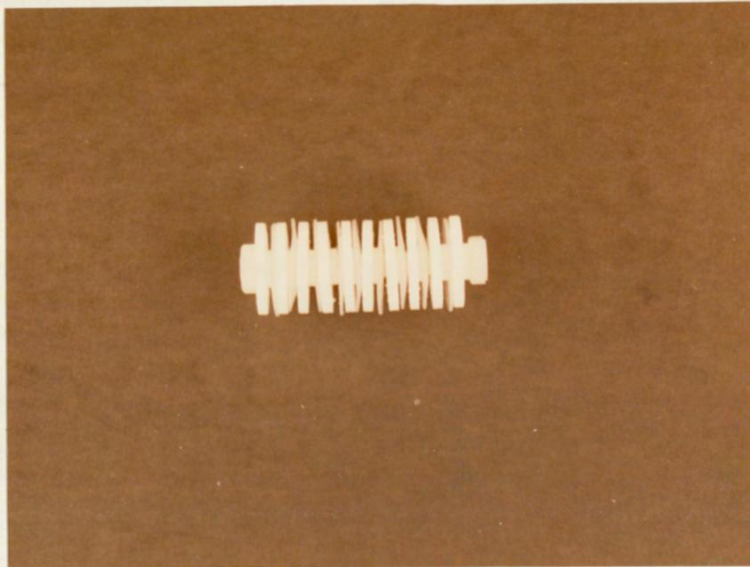
Fig. 3.2. Device implanted into rabbits in the biomaterial-associated infection model, consisting of a central rod supporting 10 discs of Silastic sheeting sandwiched between white plastic discs.
