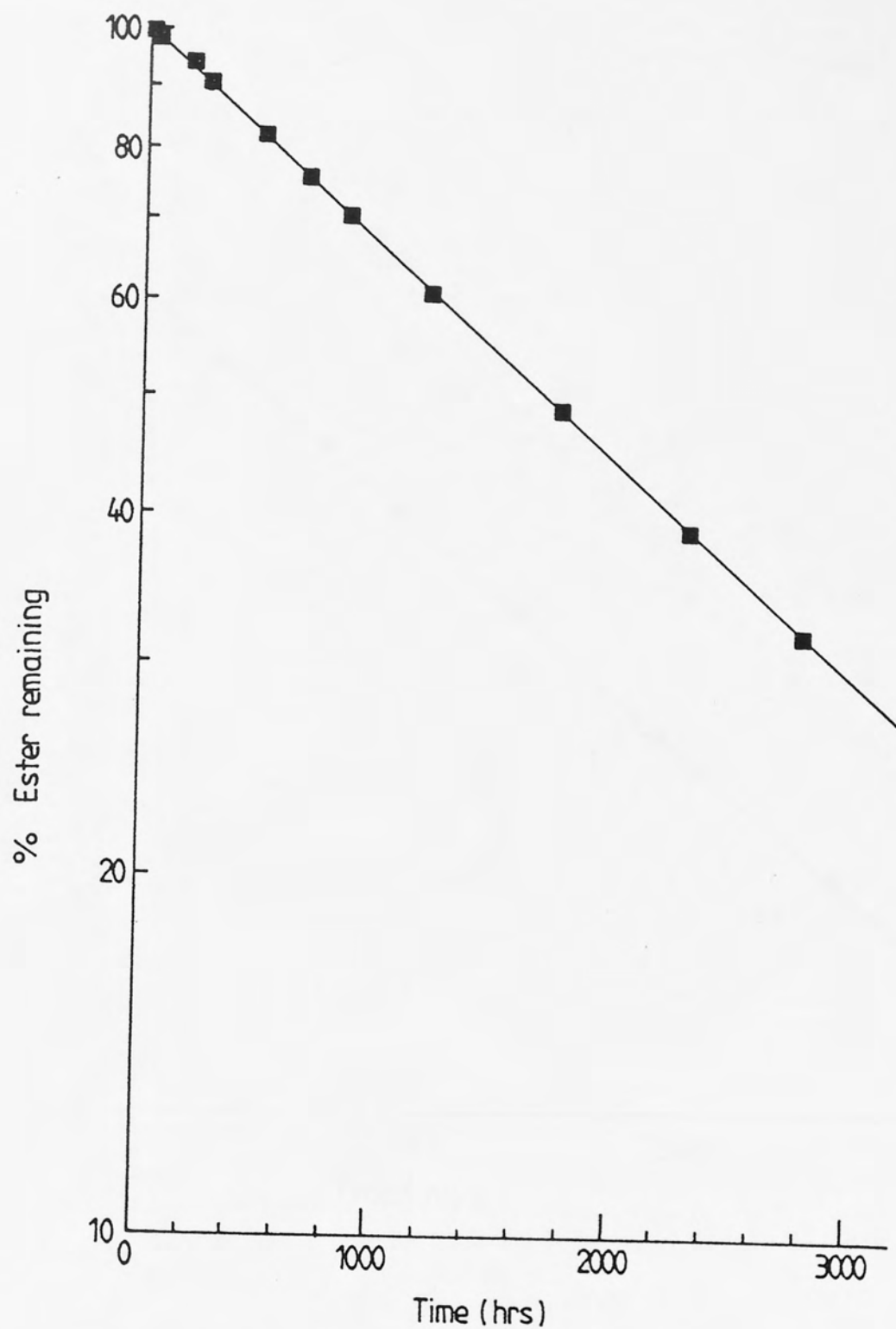
Fig. 6.3 First order plot for the hydrolysis of (tetrahydro-2-furanyl) methyl ester of ibuprofen in 20% propylene glycol -Tris buffer pH 8.14 at 37°C.
