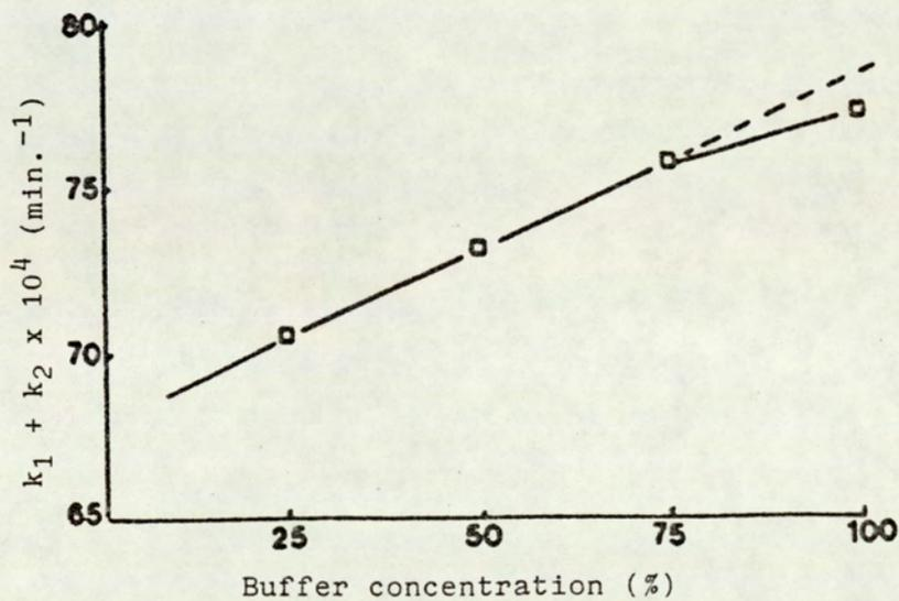
Fig 5.14 Effect of buffer concentration at pH 7.4,  $\mu = 0.5 M$  on the degradation of O-acetylpropranolol at  $37^{\circ}C$ .
