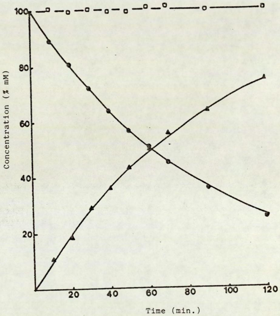
Fig 5.20 Concentration-time profile for the hydrolysis of O-pivaloylpropranolol in buffered-DMF pH 9.6 at 80°C.
