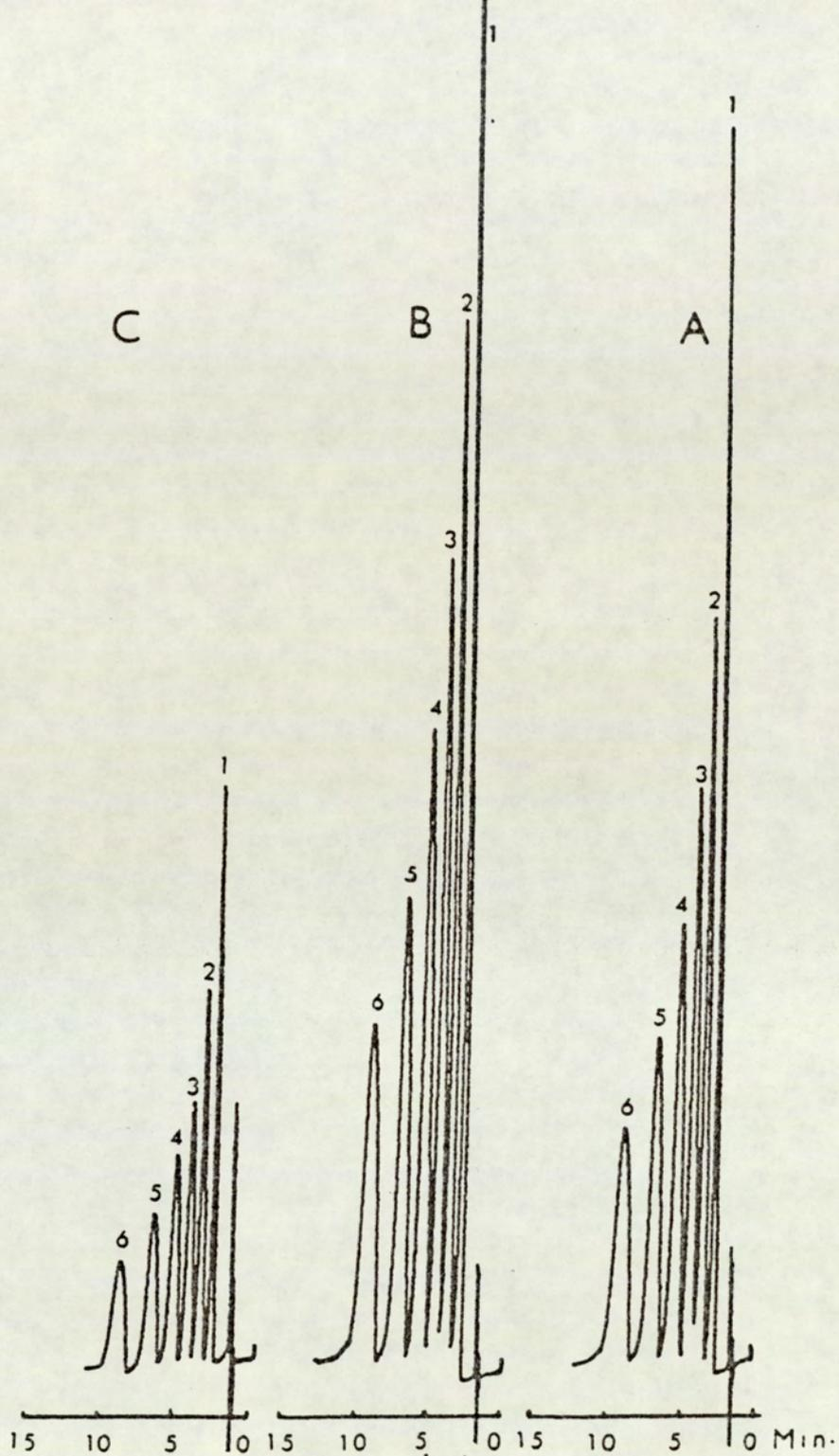
Fig 3.11 Chromatogram showing the effect of the analytical wavelength on the peak heights.
