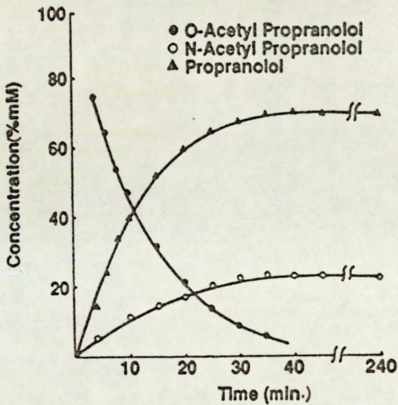
Fig 5.7 Concentration-time profile for the degradation of O-acetylpropranolol in buffered-DMF solution pH 9.45 at 80°C.
