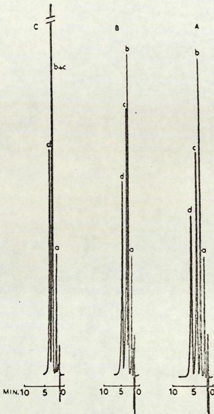
Fig 5.25 High-performance liquid chromatograms showing the effect of successive injection of a mixture of drugs in aqueous DTAB solution.
