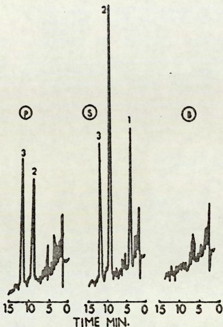
Fig 7.1 High-performance liquid chromatograms of blank plasma {B}, plasma spiked with 4-hydroxypropranolol (1), propranolol (2) and desimipramine (3) [100, 100 and 500 ng/ml respectively] {S}; and a plasma sample collected 5 hours after administration of SRP dose and supplemented with 500 ng desimipramine (Int. Std.) {P}.
