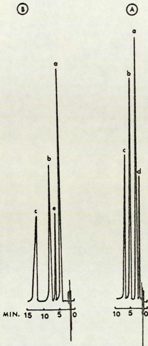
Fig 5.28 High-performance liquid chromatography of O-acetylpropranolol in buffered-surfactant pH 7.4 at 37°C. (initial concentration 0.2 mM)
