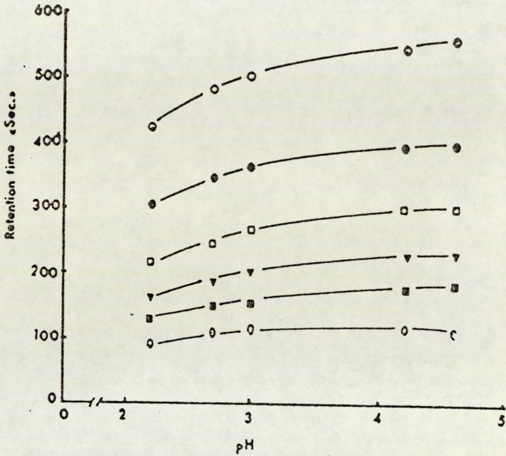
Fig 3.8 Graphical Presentation showing the Effect of the Mobile Phase pH on the Retention Time
