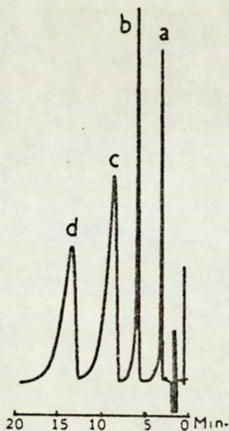
Fig 3.3 HPLC Separation of Ethyl Paraben as an Internal Standard (a), N,O-diacetylpropranolol (b), Propranolol (c) and O-acetylpropranolol (d).
