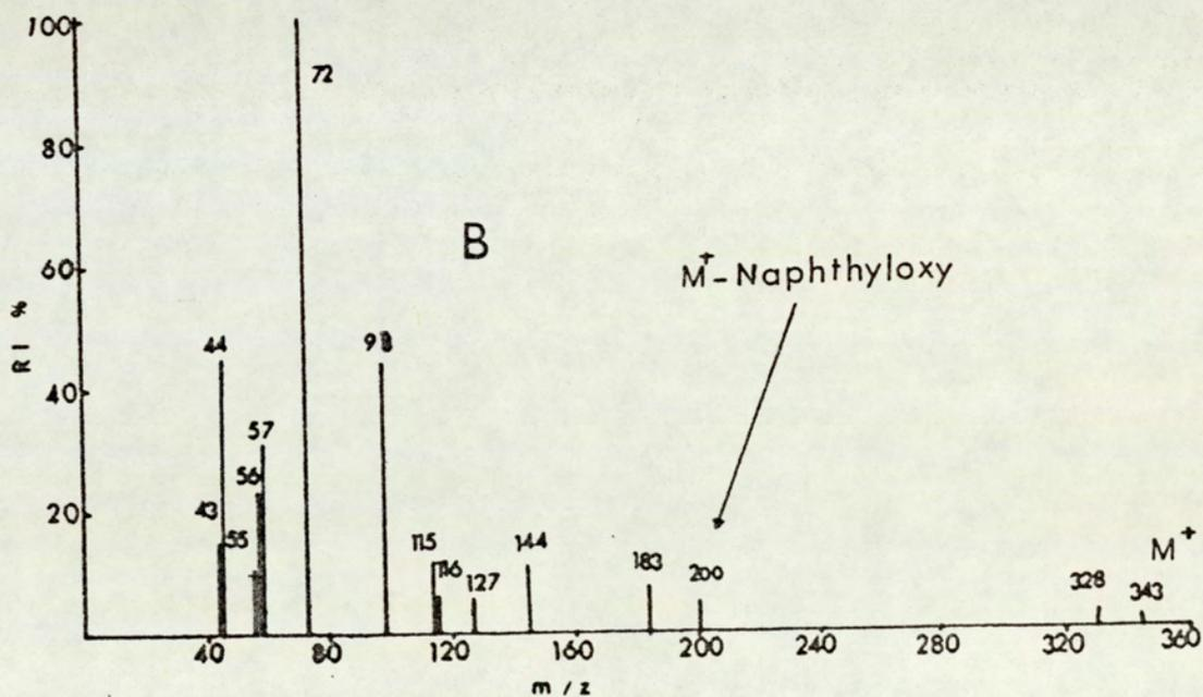
Appendix IV.5 Mass Spectral Fragmentation of N-O-diacetylpropranolol (A), and O-pivaloylpropranolol (B).
