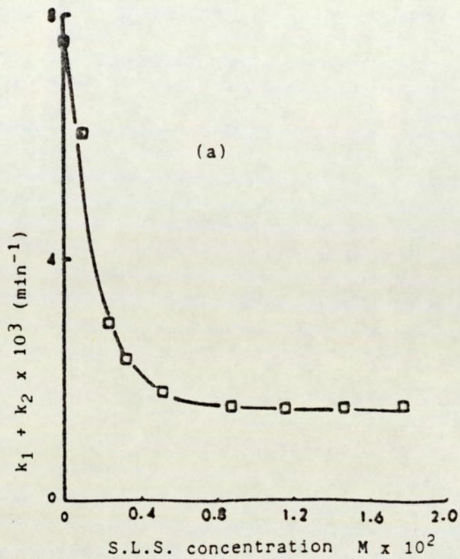
Fig 5.33 (a) Effect of sodium lauryl sulphate (SLS) concentration on the degradation of O-acetylpropranolol in buffer pH 7.4,  $\mu = 0.5M$  at 37°C.
