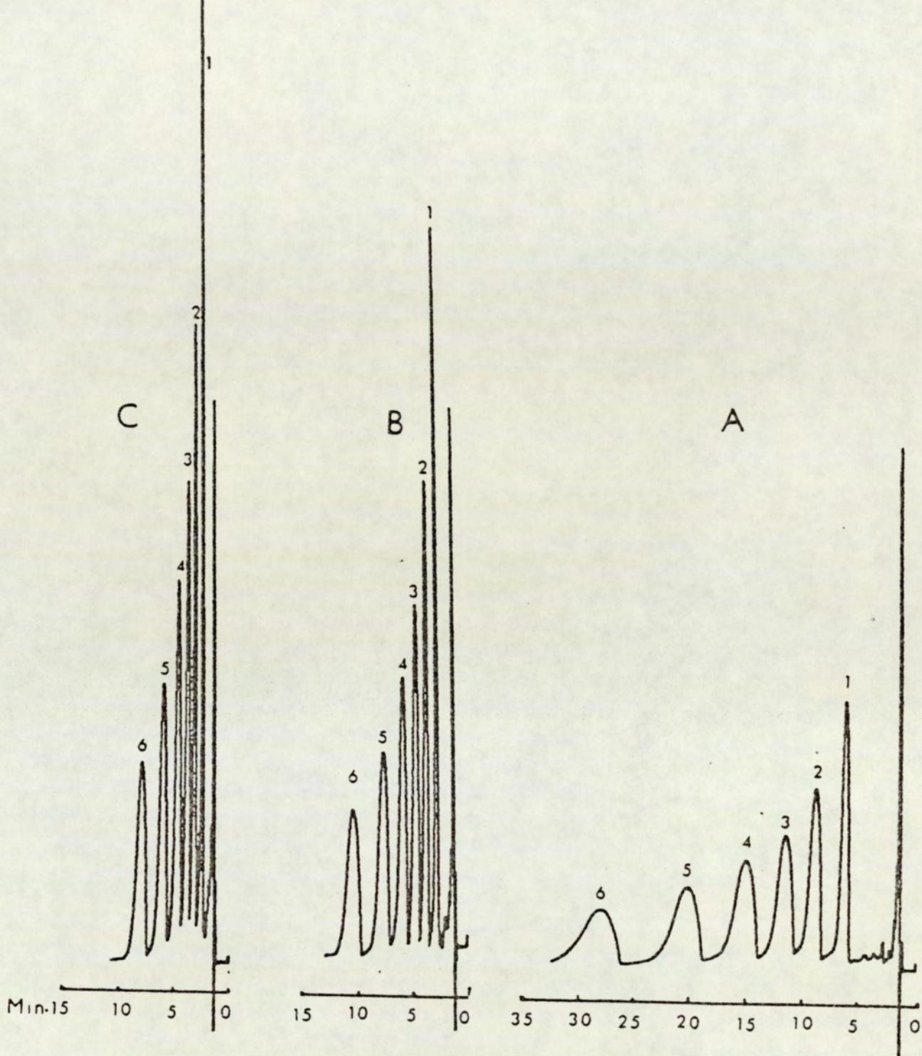
Fig 3.6 Chromatogram showing the effect of the Diethylamine proportion in the mobile phase on the elution of Beta-blockers.
