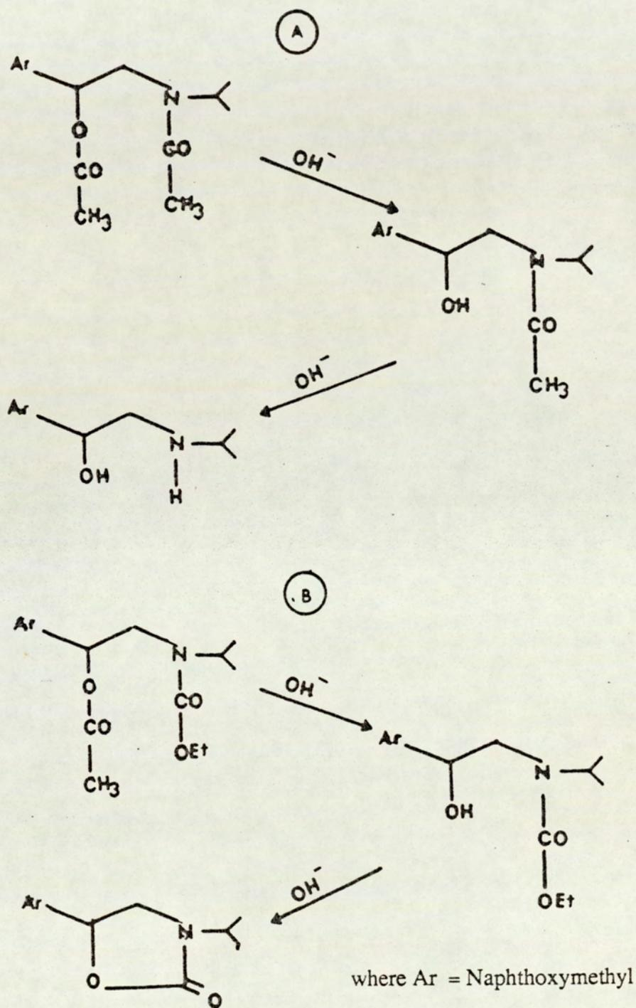
Fig 5.41 Models showing the possible route of degradation of N, O-diacetylpropranolol (A) and N-ethoxycarbonyl, O-acetylpropranolol (B) in alkaline DMF (50% v/v, 0.25M NaOH) at 37°C.
