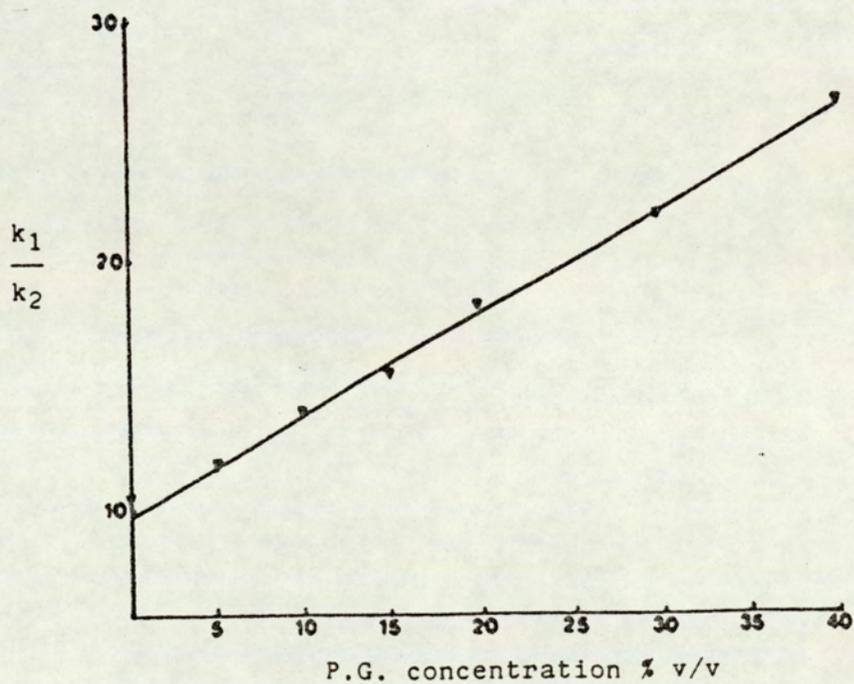
Fig 5.18 Effect of P.G. Concentration on  $k_1/k_2$  for the degradation of O-acetylpropranolol in buffer pH 7.4 at 37°C.
