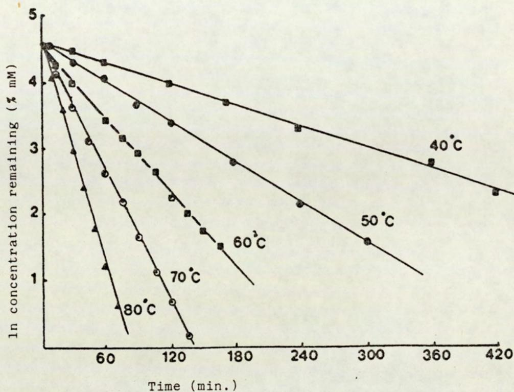
Fig 5.23 Ln concentration of O-pivaloylpropranolol at various temperatures in buffered-DMF pH 9.6.
