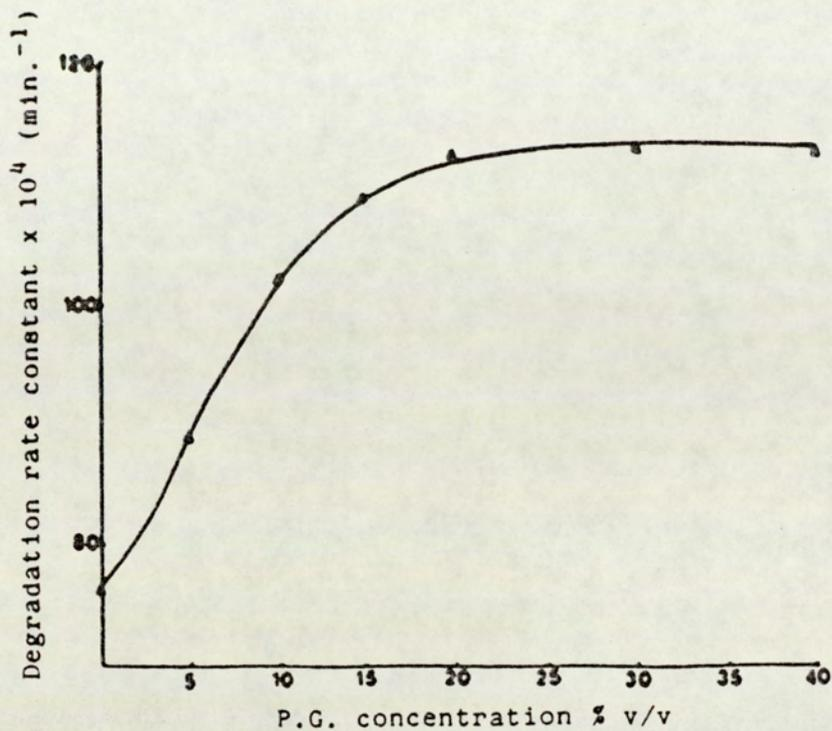
Fig 5.17 Effect of propylene glycol (P.G.) concentration on the degradation of O-acetylpropranolol in buffer pH 7.4 at 37°C.
