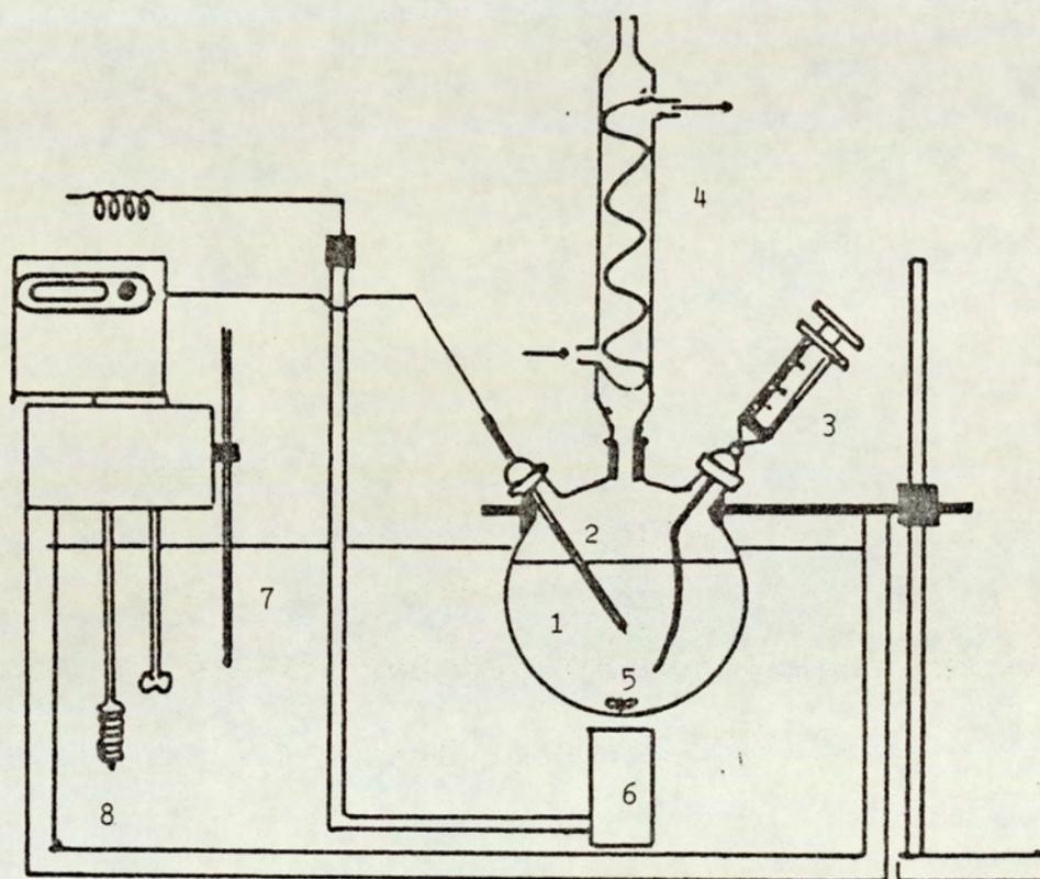
Fig 5.1 (a) Block diagram of the equipment used for the stability kinetics studies.
