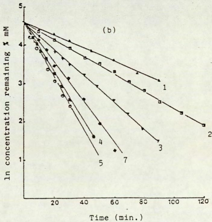
Fig 5.36 First-order plots showing the effect of the side chain on the enzymatic degradation of O-acyl propranolol (a) in isolated esterase (b) in serum. The numbers indicate the number of carbon atoms in the ester side chain.
