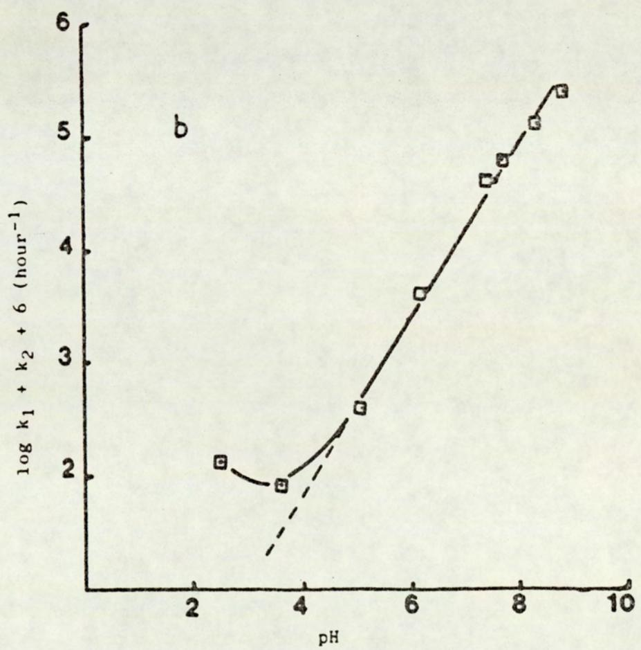
Fig 5.5 pH - rate profiles for the degradation of (a) O-acetyl and (b) O-hexanoyl propranolols in buffered-DMF solutions at various pH values at 80°C.
