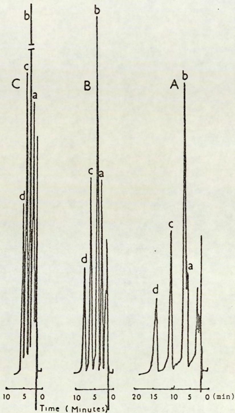
Fig 3.4 Chromatograms showing the effect of the Acetonitrile proportion in the mobile phase on the separation of N-acetylpropranolol (a), Propranolol (b), O-acetylpropranolol (c) and O-propionylpropranolol (d).
