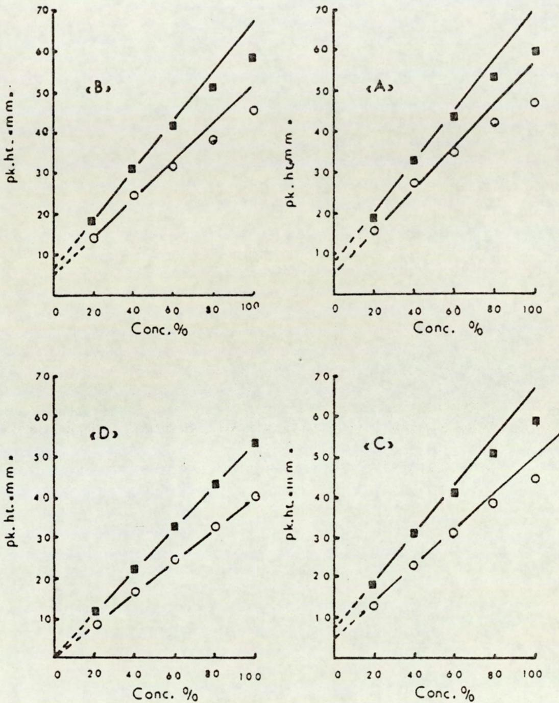
Fig 3.12 Effect of DMF Concentration on the linearity of the Calibration Curve for O-pivaloylpropranolol ( ■ ) and O-hexanoylpropranolol ( ○ ).
