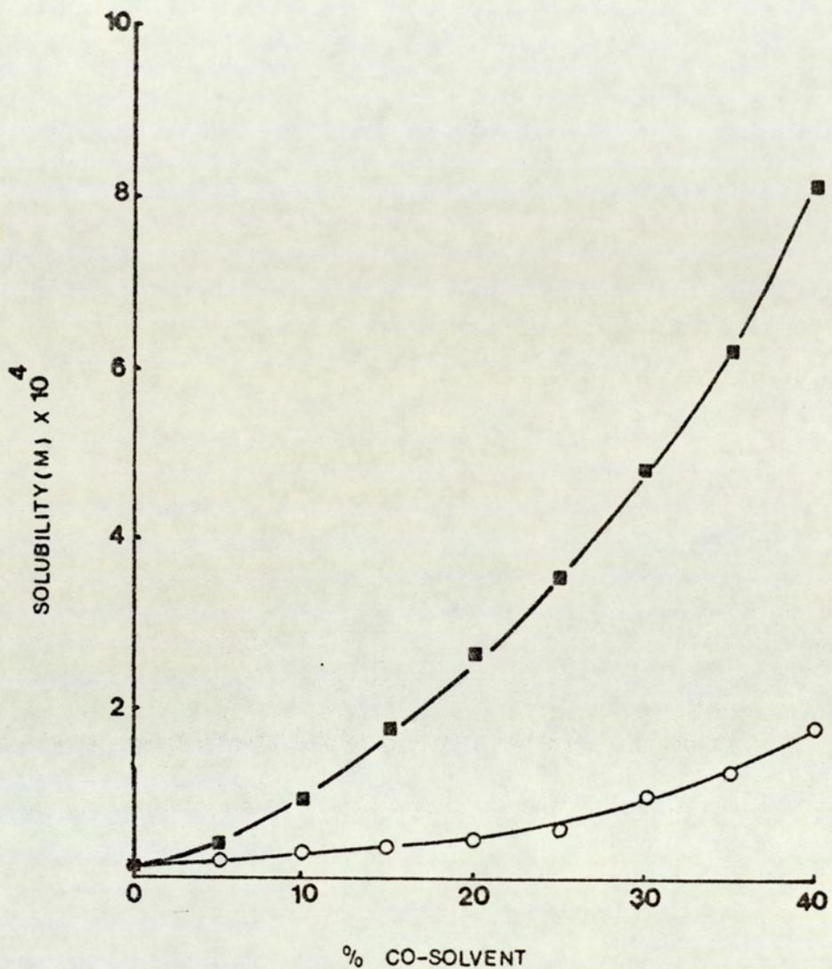
Fig 4.12 Solubility of N,O-diacetylpropranolol in DMF-buffer mixtures (■) and in P.G.-buffer mixtures (○).
