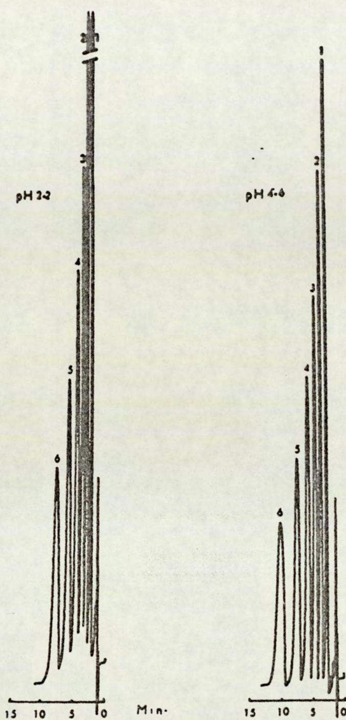
Fig 3.9 Comparative Chromatograms showing the effect of the Mobile Phase pH on the Elution of Beta-blockers.
