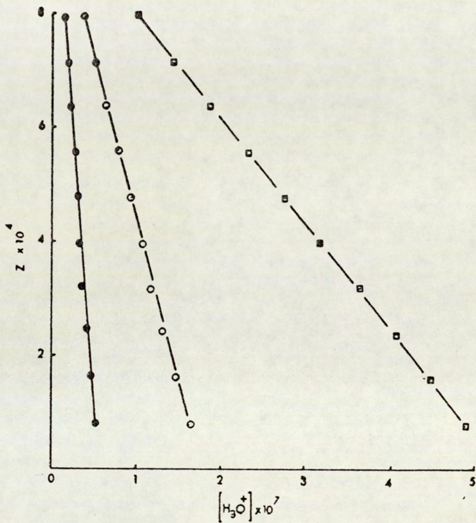
Fig 4.9 Non-logarithmic titration of O-hexanoylpropranolol ( $\square$ ), O-valerylpropranolol ( $\circ$ ) and O-butyrylpropranolol ( $\bullet$ ).
