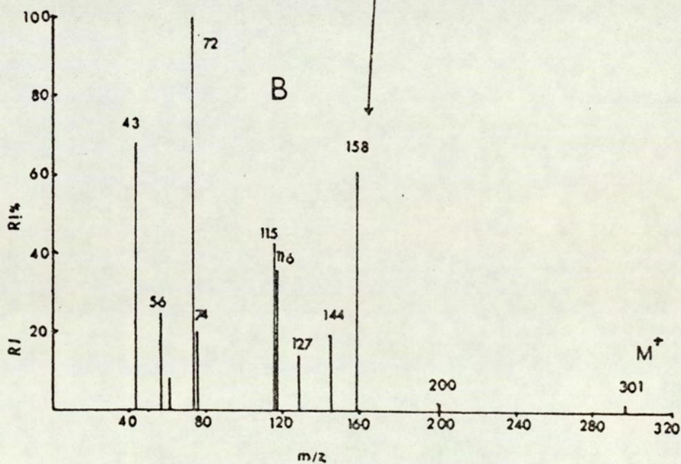
Appendix IV.1 Mass Spectral Fragmentation of O-acetylpropranolol (A), and N-acetylpropranolol (B).
