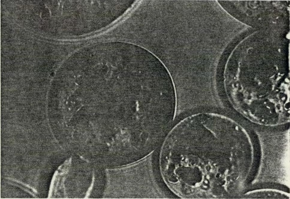
Fig 6.20 Microencapsulated Propranolol resin (IRP69) complex after Dissolution (X400)
