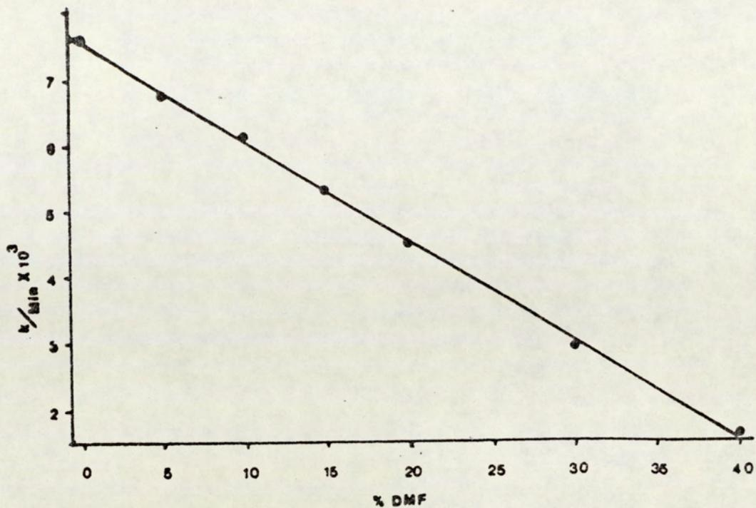
Fig 5.15 Effect of DMF concentration on the degradation of O-acetylpropranolol in buffer pH 7.4 at 37°C.
