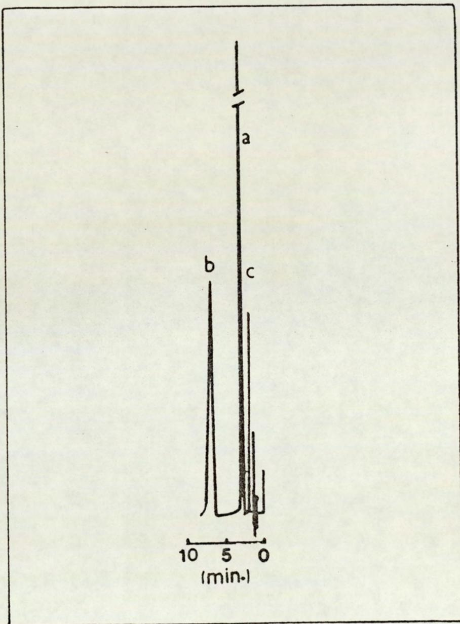
Fig 6.2 Chromatogram showing the separation of propranolol (a) O-pivaloylpropranolol (b) and ethyl paraben as internal standard (c) using a mobile phase consisted of acetonitrile, orthophosphoric acid (88%), diethylamine and water (65:0.1:0.2:34.7) at flow rate 1 ml/min, detection at 290 nm.
