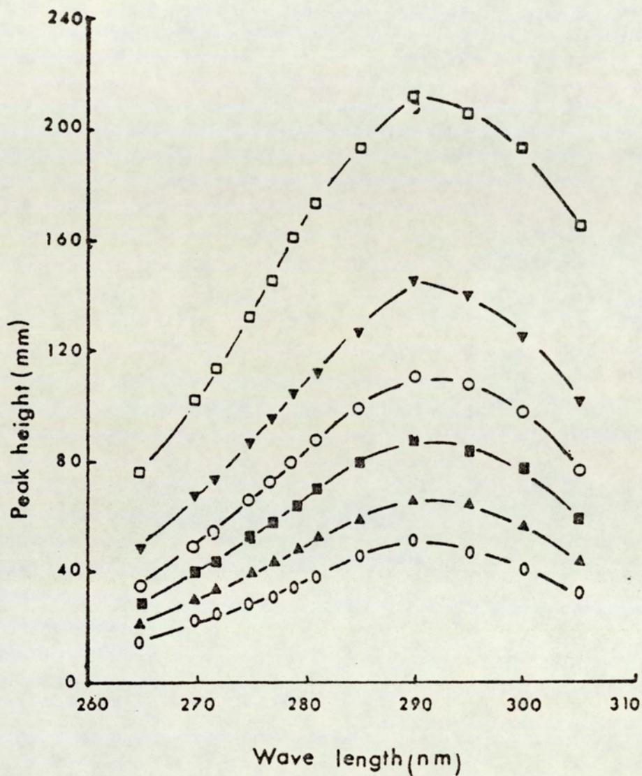
Fig 3.10 Effect of the Analytical Wavelength on the Peak Height
