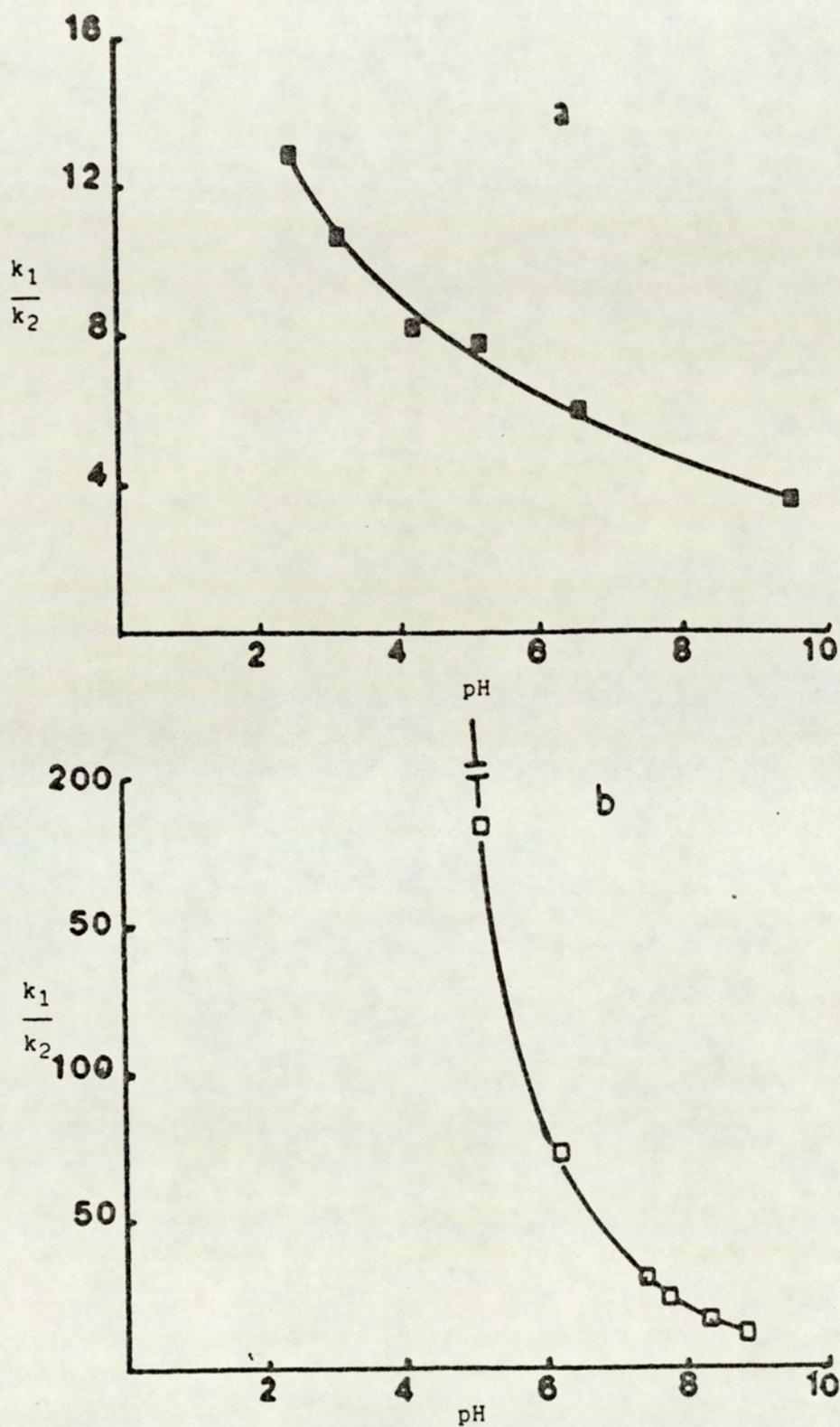
Fig 5.9 Effect of pH on  $k_1/k_2$  ratios for the degradation of (a) O-acetyl and (b) O-hexanoyl propranolols in buffered-DMF solutions at various pH values at 80°C.
