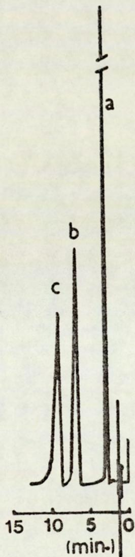
Fig 3.13 Chromatogram Showing the Separation of Propranolol (a), O-pivaloylpropranolol (b), and O-hexanoylpropranolol (c), using a Mobile Phase (System II) at Flow Rate 1ml/min, Detection at 290 nm.
