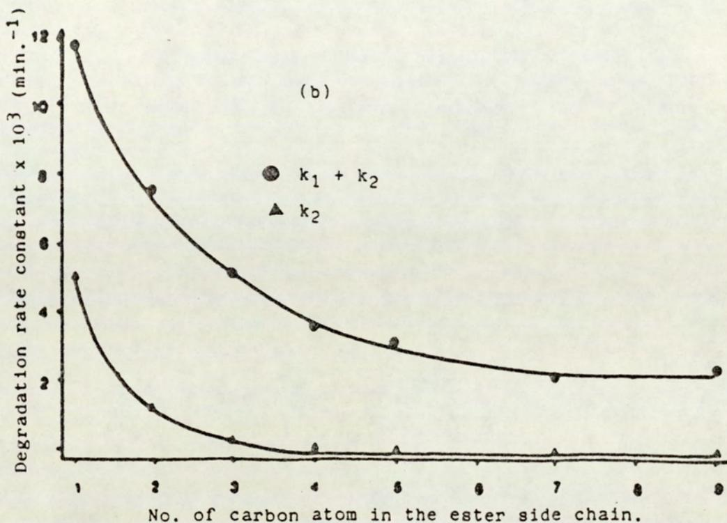
Fig 5.4 (b) Effect of the ester side chain on the degradation of propranolol esters in buffered-DMF pH 10 at 37°C.
