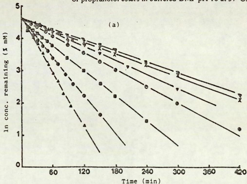
Fig 5.4 (a) ln concentration time profile for the degradation of O-acyl propranolols in buffered-DMF pH 10 at 37°C.
