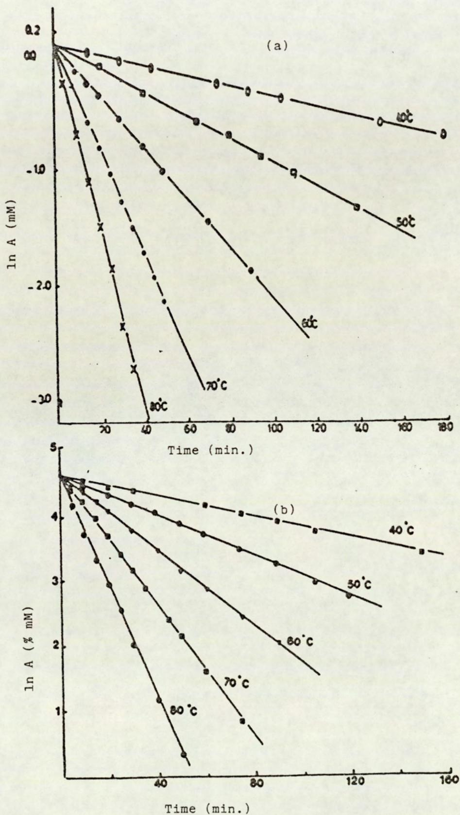
Fig 5.10 Ln of concentration of O-acetylpropranolol (a) and O-hexanoylpropranolol (b) against time at various temperatures in buffered-DMF solutions pH 9.45 and 10.7 respectively.
