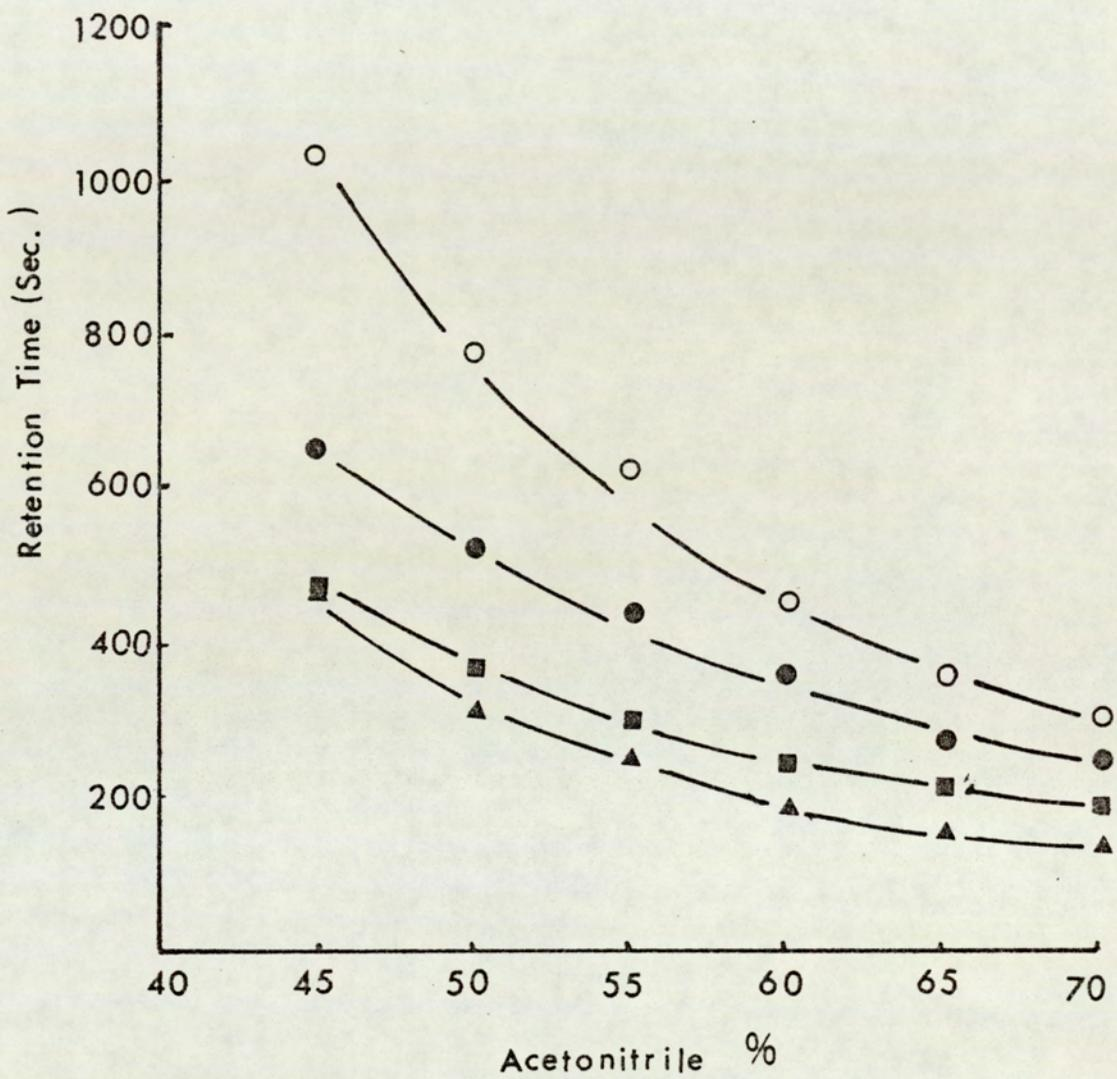
Fig 3.5 Effect of Acetonitrile % in the Mobile Phase on the Retention Time of N-acetylpropranolol (▲), Propranolol (■), O-acetylpropranolol (●) and O-propionylpropranolol (○).
