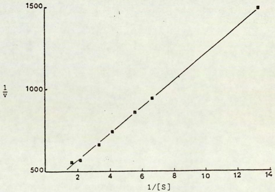
Fig 5.39 (b) Lineweaver-Burk plot for the hydrolysis of O-pivaloylpropranolol in presence of 120 units of esterase in 10% buffered-DMF pH 7.4 at 37°C.
