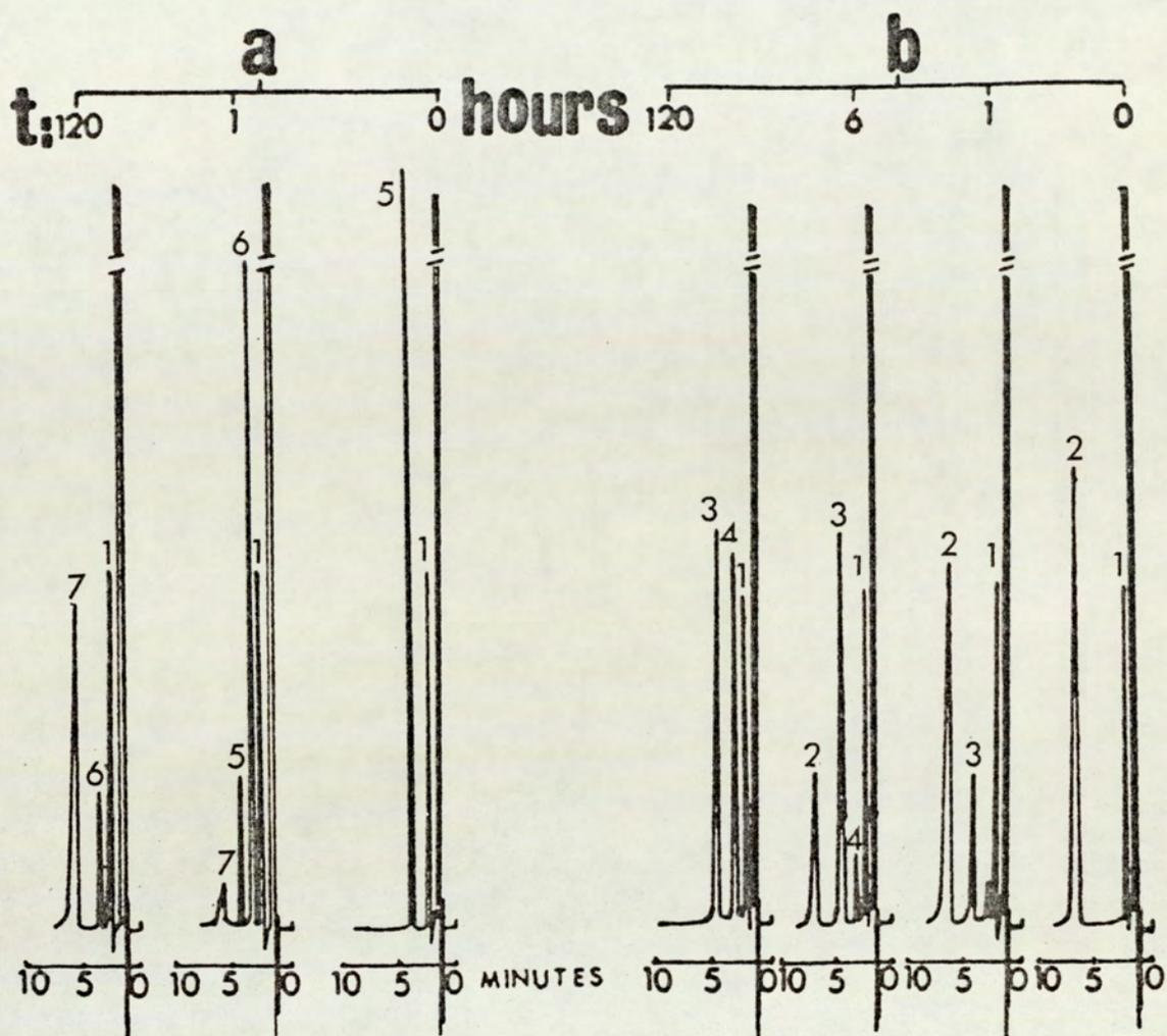
Fig 5.40 High-performance liquid chromatograms showing the degradation of N, O-diacetylpropranolol (a) and N-ethoxycarbonyl, O-acetylpropranolol (b) in alkaline DMF (50% v/v, 0.25 M NaOH) at 37°C.
