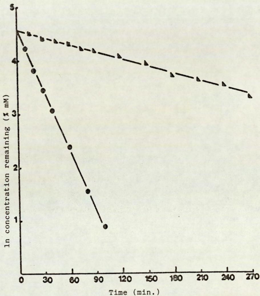
Fig 5.43 First-order plots of the degradation of N,O-diacetylpropranolol (●) and N,ethoxycarbonyl, O-acetylpropranolol (▲) in alkaline DMF (50%, 0.25 M NaOH) at 37°C.
