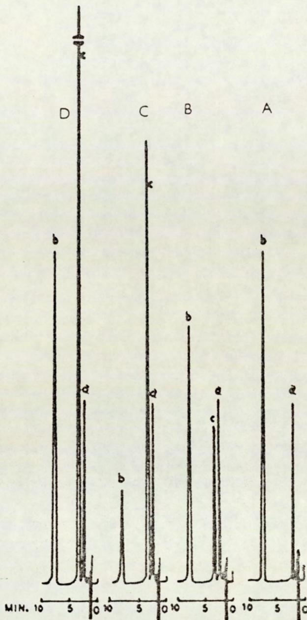
Fig 5.19 High-performance liquid chromatogram showing the hydrolysis of O-pivaloylpropranolol (0.5 mM) in buffered-DMF solution pH 9.6 at 80°C.
