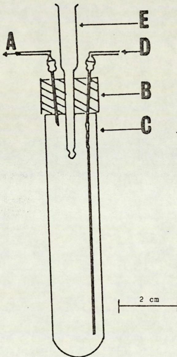
Fig 5.1 (b) Diagrammatic representation of the apparatus used for the study of the degradation of propranolol esters during absorption.
