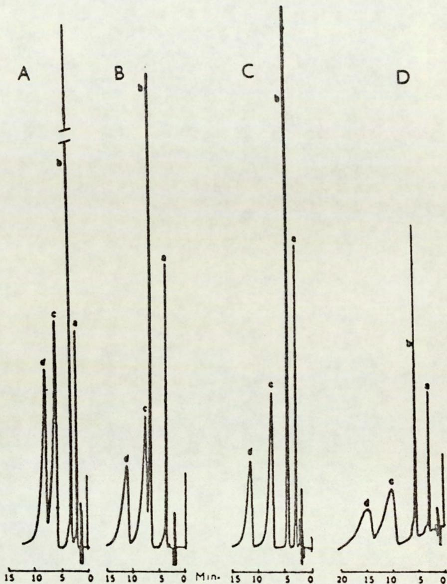
Fig 3.2 Development of the HPLC Separation for Ethyl Paraben as Internal Standard (a), N-acetylpropranolol (b), Propranolol HCl (c) and O-acetylpropranolol (d).
