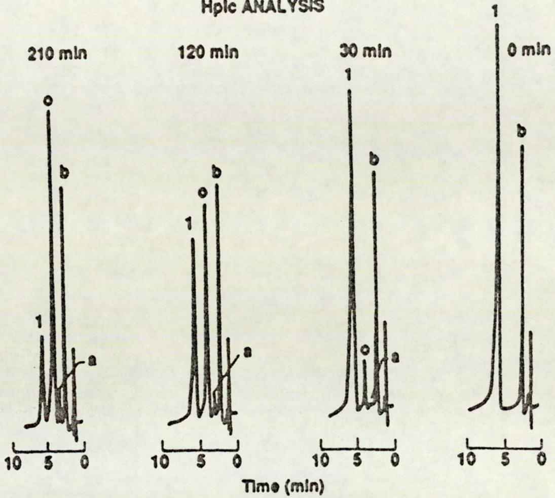
Fig 5.8 High-performance liquid chromatograms of the degradation of O-acetylpropranolol in buffered-DMF solution pH 9.45 at 80°C.
