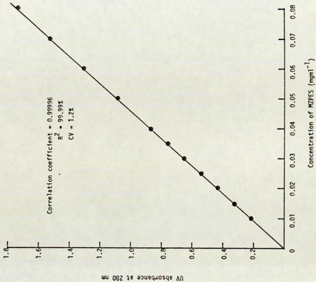
Fig. 8. HPLC Peak Height ratio MZPES/Pyrimethamine (Internal standard) Vs Concentration of MZPES
