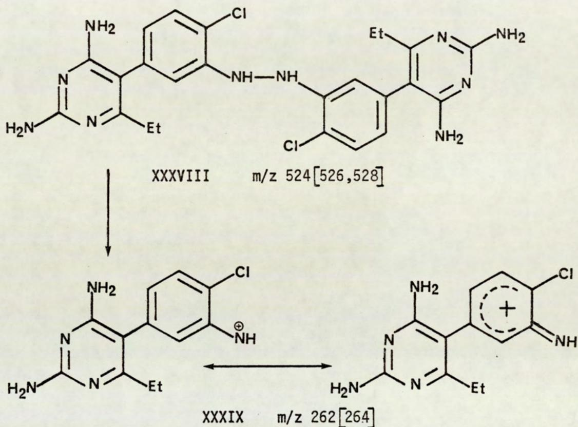
Scheme 13. Expected fragmentation of 5,5'-bis(2,4-diamino-6-ethylpyrimidin-5-yl)-2,2'-dichlorohydrazobenzene in mass spectrometry.
