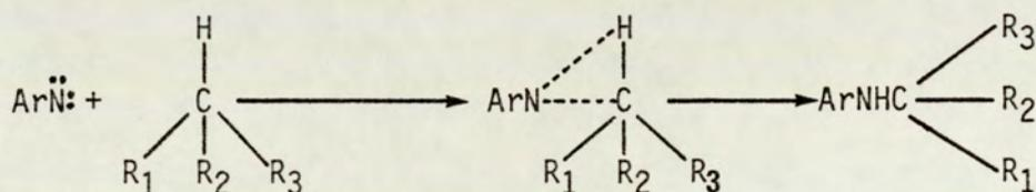
Scheme 4. Insertion of singlet nitrene into C-H bond
