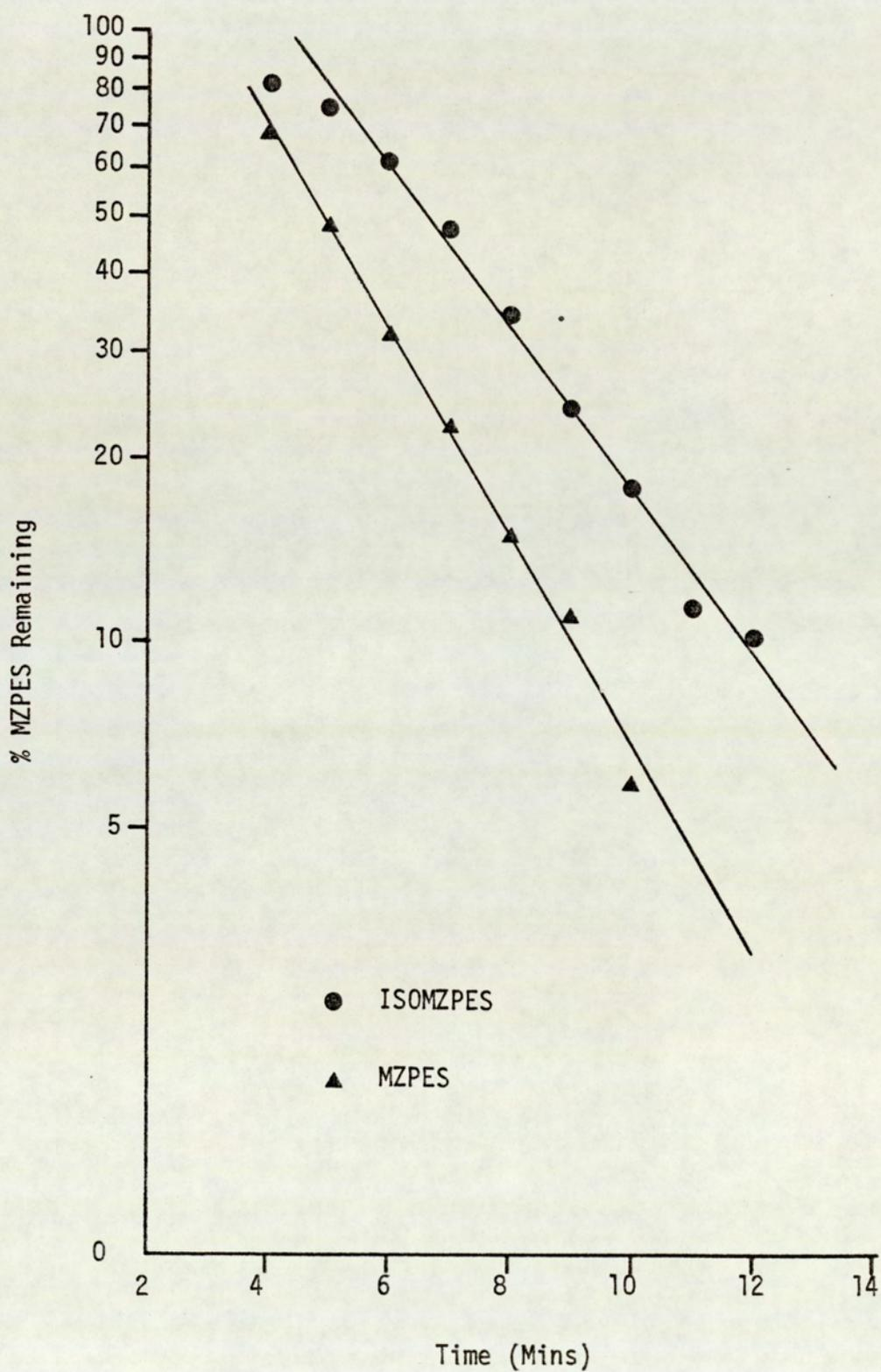
Fig. 31. Photolysis of ISOMZPES in oxygen-saturated water
