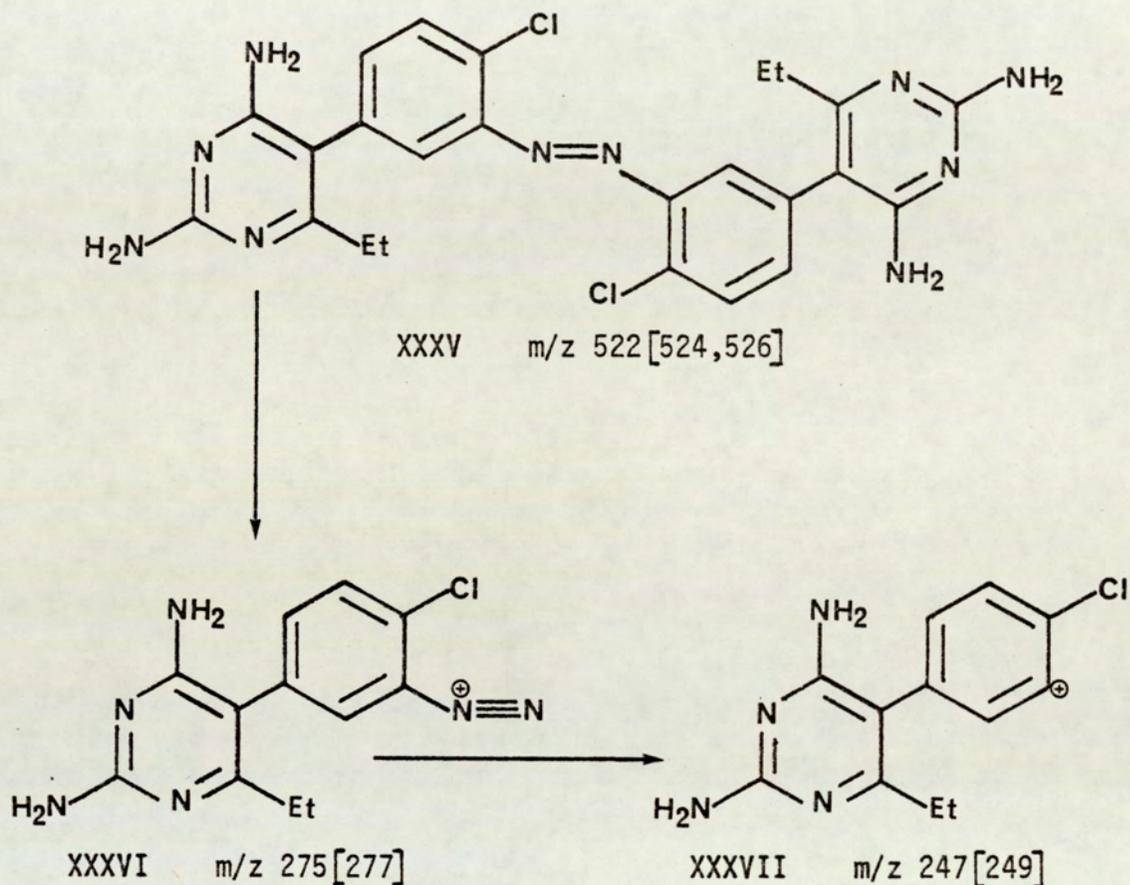
Scheme 12 Expected fragmentation of 5,5'-bis(2,4-diamino-6-ethylpyrimidin-5-yl)-2,2'-dichloroazobenzene in mass spectrometry.
