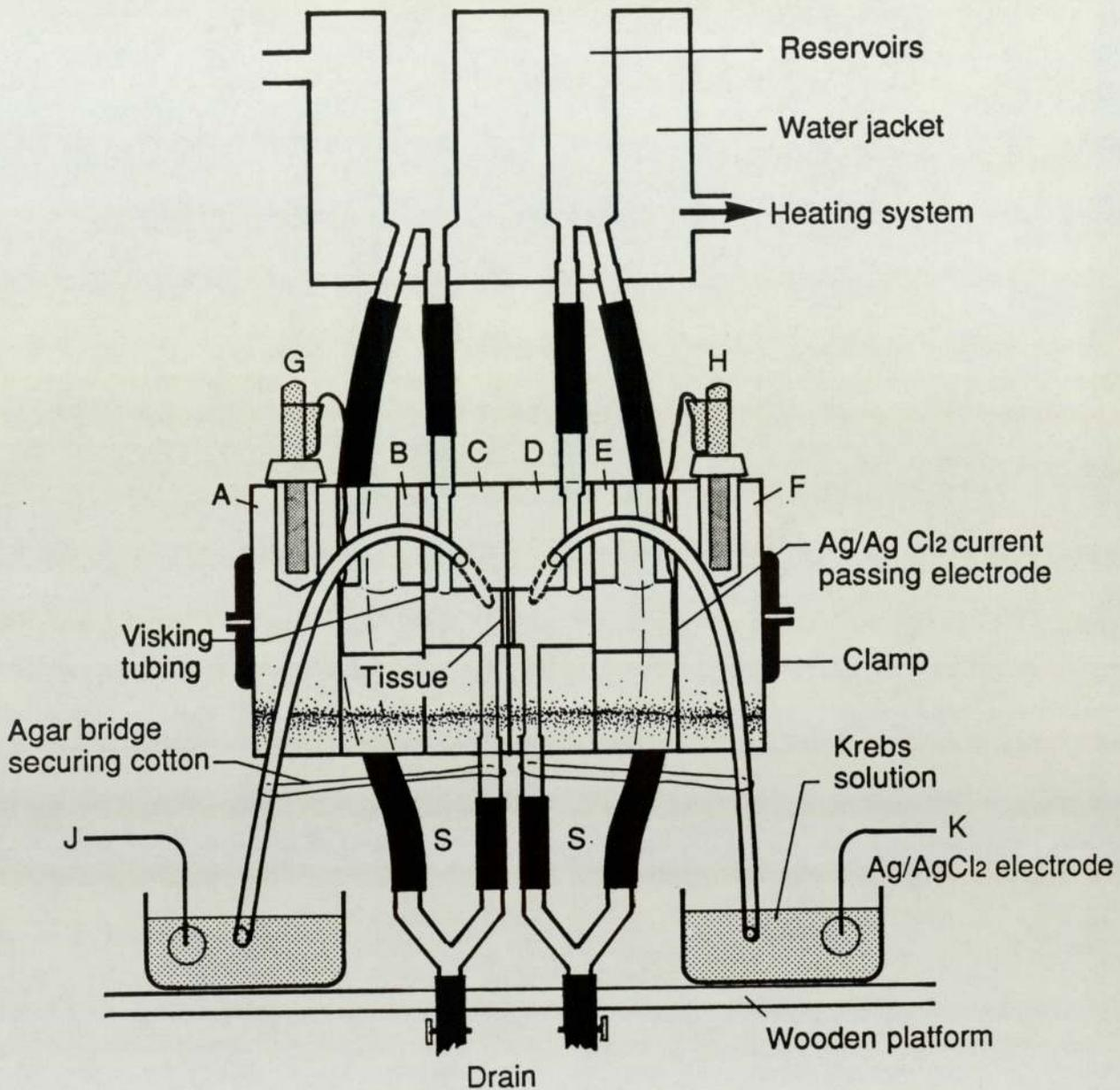
Fig. 2. Diagrammatic representation of type I Ussing chambers. The chamber system consisted of 6 interlocking perspex discs (A-F) connected to water jacketed reservoirs via siliconised rubber tubing. G, H, I, J represent references for electrode connections (see text for details). At the points (S) syringe needles leading from a 95% O<sub>2</sub>/5% CO<sub>2</sub> supply were inserted into the rubber tubing to provide oxygenation and gas lift circulation.
