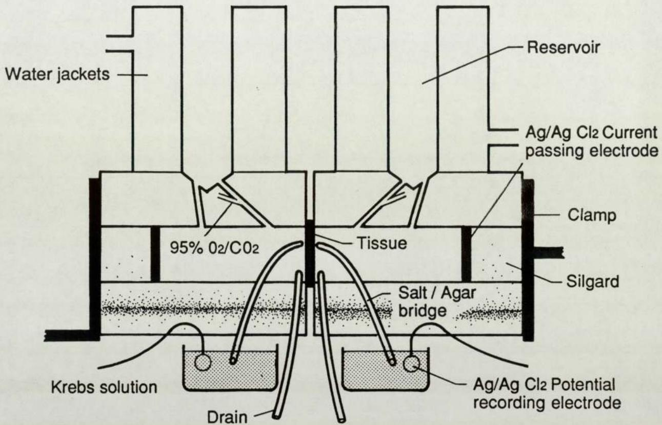
Fig. 3. Diagrammatic representation of type II Ussing chambers. The system comprised of two interlocking perspex half chambers with bathing fluid reservoirs and water jackets actually mounted on top of the chambers (see text for details).
