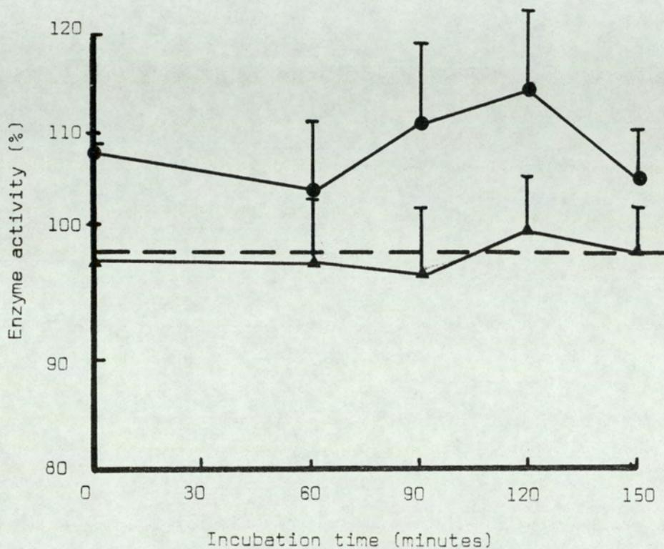
Fig. 53. Stability of free AP (●) and NAG (▲) during incubation at 37°C for up to 2.5 hours in the presence of  $10^{-3}$  M gentamicin. Activities at each time are expressed as a percentage of the control activity at that time which is set to 100%. Each point is the mean  $\pm$  s.e.m. of two experiments each done in triplicate.
