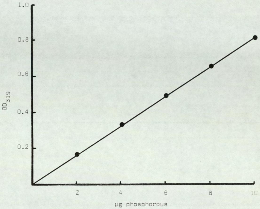
Fig. 12. Calibration curve of Pi by the modified method of Ueda and Wada, with the addition of methanol. The readings were identical in the absence and presence of gentamicin ( $10^{-2}$  M).
