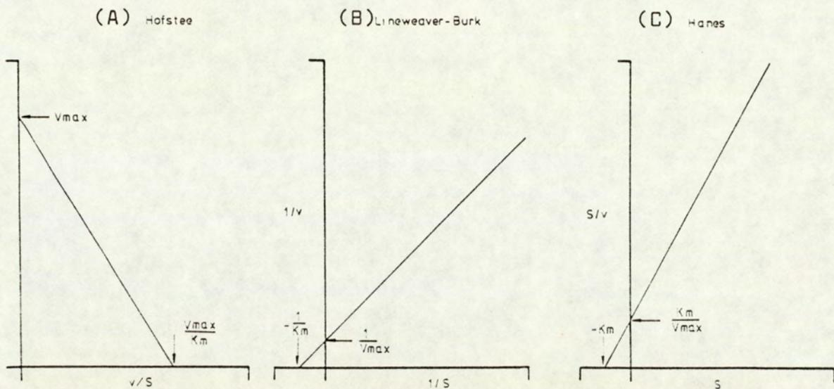
Fig. 5. Graphical methods for the determination of the kinetic constants,  $K_m$  and  $V_{max}$ . Each plot represents a linear transform of the Michaelis-Menten equation devised by (A) Hofstee (1959), (B) Lineweaver and Burke (1934) and (C) Hanes (1932). Initial velocity is represented by ( $v$ ) and substrate concentration by ( $S$ ).
