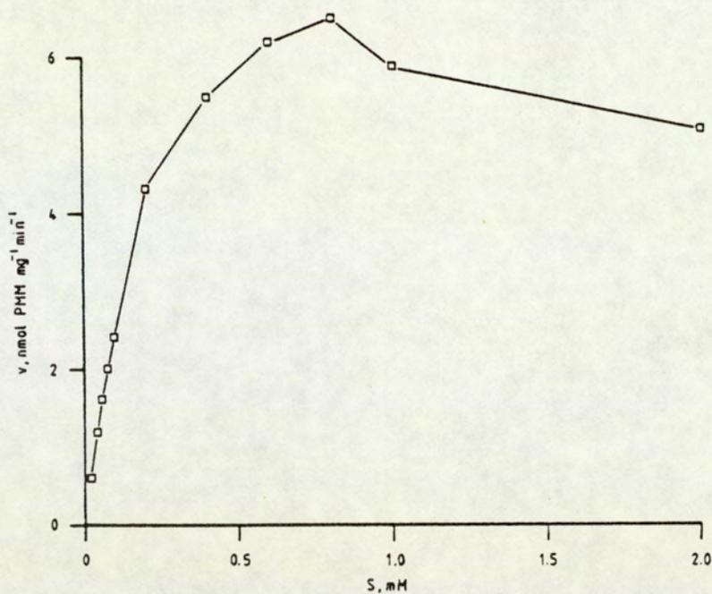
Fig. 16 Inhibition of the in-vitro metabolism of HMM at substrate concentrations above 0.5 mM. The appearance of the N-demethylated metabolite (PMM) was estimated by GC. Initial velocities ( $v$ ) are plotted against substrate concentration ( $S$ ). Experimental points are the means of three determinations.
