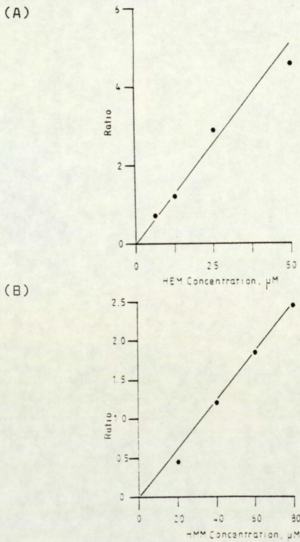
Fig. 9. The linearity of the GC detector response (peak height ratio) with various concentrations of HEM (A) and HMM (B). Each value is the mean of duplicate determinations from one experiment.
