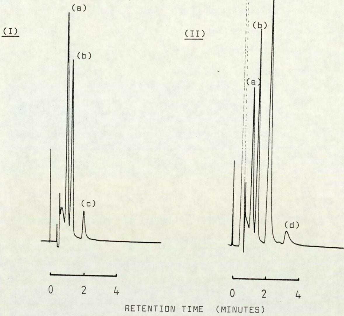
Fig. 33C Gas chromatograms of plasma (I) and urine (II) samples obtained from one mouse after IP administration of 496.4 mg/Kg DMF. Plasma and urine samples were obtained two hours and six hours after drug administration respectively. Peaks (a), (b), (c) and (d) correspond to DMF, TMU (30  $\mu\text{g/ml}$ ), NMF and formamide respectively.
