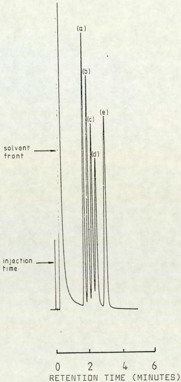
Fig. 10 Gas chromatogram of a standard solution of the N-alkylmelamines by flame ionization detection. HMM (a), PMM (b), TetraMM (c), TriMM (d) and HEM (e) were dissolved in acetone to give a concentration of  $50\mu\text{M}$ .
