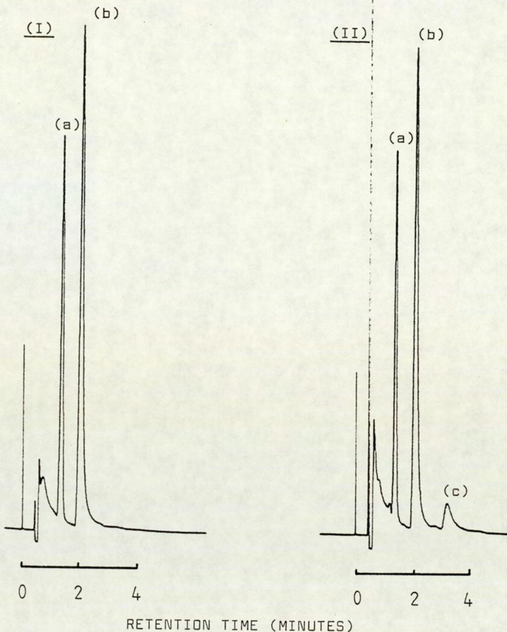
Fig. 33A Gas chromatograms of mouse plasma (I) and urine (II) after IP administration of 400 mg/Kg NMF. Plasma and urine samples were obtained 2 hours and 6 hours after drug administration respectively, and treated according to section (8.3.1). Peaks (a), (b) and (c) correspond to TMU (30  $\mu\text{g}/\text{ml}$ ), NMF and formamide respectively.
