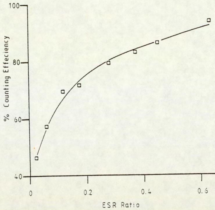
Fig. 29 Correlation curve between the sample counting efficiency and the count rate of the external standard. (External standard ratio; ESR).
