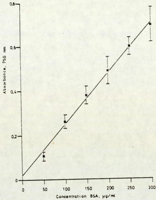
Fig. 3. Standard curve for the estimation of protein concentration.
