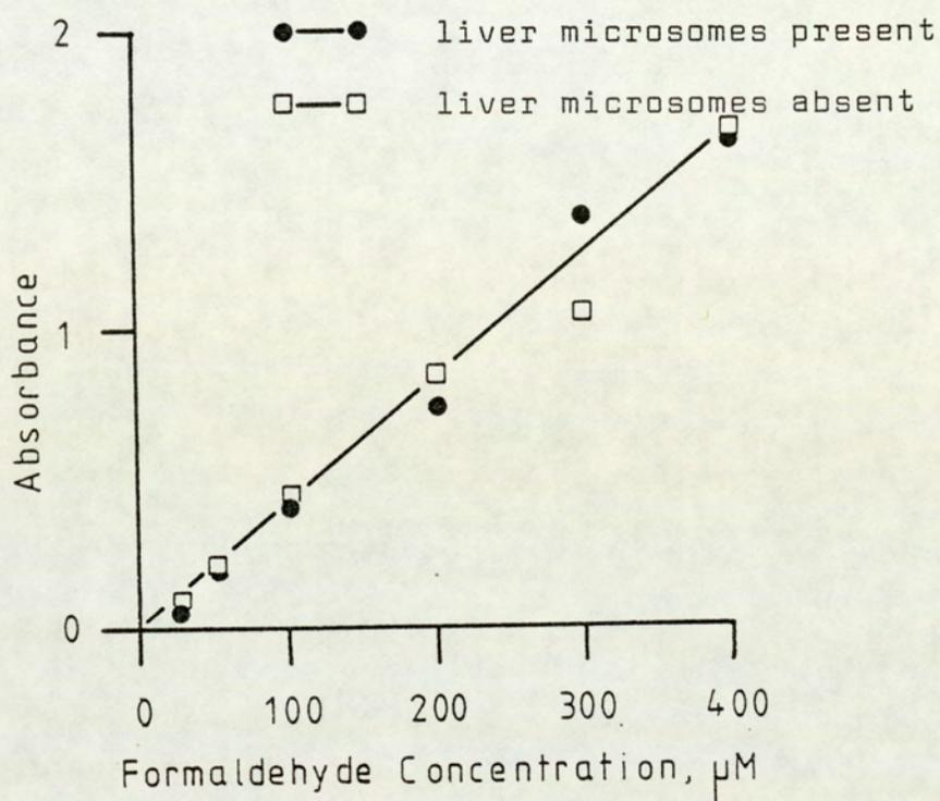
Fig. 8 The effect of addition of mouse liver microsomes (2mg protein/ml) on the absorbance of various formaldehyde concentrations. Absorbance was measured at 412nm in the presence (●—●) and absence (□—□) of liver microsomes. Each value is the mean of duplicate determinations from one experiment.
