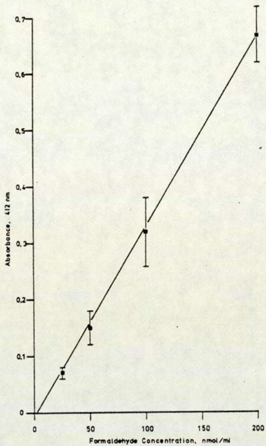
Fig. 4 Calibration curve for the estimation of formaldehyde. The absorbance of various formaldehyde solutions at 412 nm.
