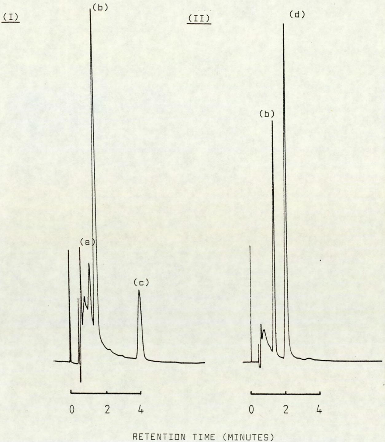
Fig. 33D Gas chromatograms of mouse plasma obtained two hours after IP administration of 100 mg/Kg DMSF (I) and 591 mg/Kg NEF (II). Peaks (a), (b), (c) and (d) correspond to DMF, TMU (30  $\mu\text{g/ml}$ ), DMSF and NEF respectively.
