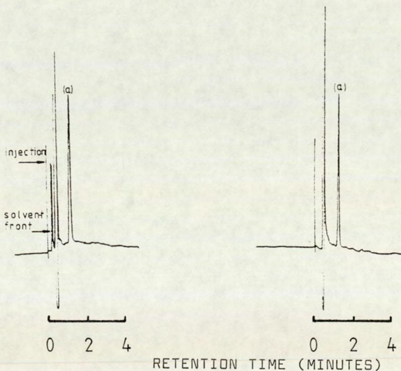
Fig. 32 Gas chromatograms of mouse (I) and patient (C.R.) (II) plasma (on the left) and urine (on the right), before administration of drug. (a) corresponds to the internal standard (TMU). Samples were prepared and treated according to section (8.3.1).
