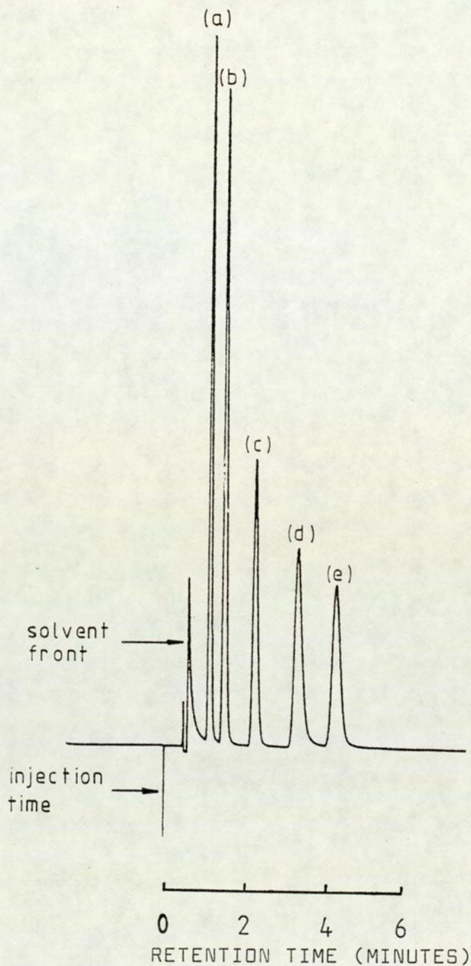
Fig. 30 Gas chromatogram of a standard solution of the N-alkylformamides by nitrogen-phosphorus detection. DMF (a), TMU (b), NMF (c), formamide (d) and DMSF (e) were dissolved in acetone to give a final concentration of  $30\mu\text{g/ml}$ .
