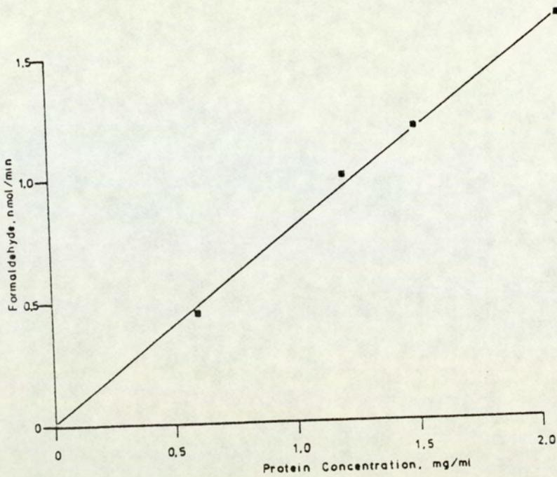
Fig. 7. Linearity of formaldehyde formation, from the N-demethylation of HMM, with the concentration of microsomal protein (0.6-2.1mg/ml). Incubations contained 2mM HMM and were terminated after 20 minutes. Each value is the mean of duplicate determinations from one experiment.
