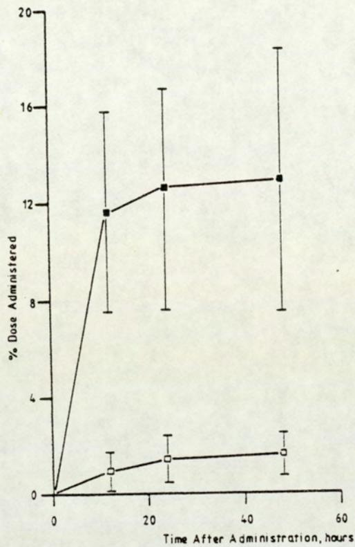
Fig. 52 Cumulative urinary excretion of NMF (■) and formamide (□) after IP administration of 400 mg/Kg NMF where samples were obtained without washing the metabolic cages. Values are expressed as % of the dose administered and are the mean ( $\pm$  s.d.) of three determinations. There are no measurable levels of unchanged NMF or formamide after 48 hours.
