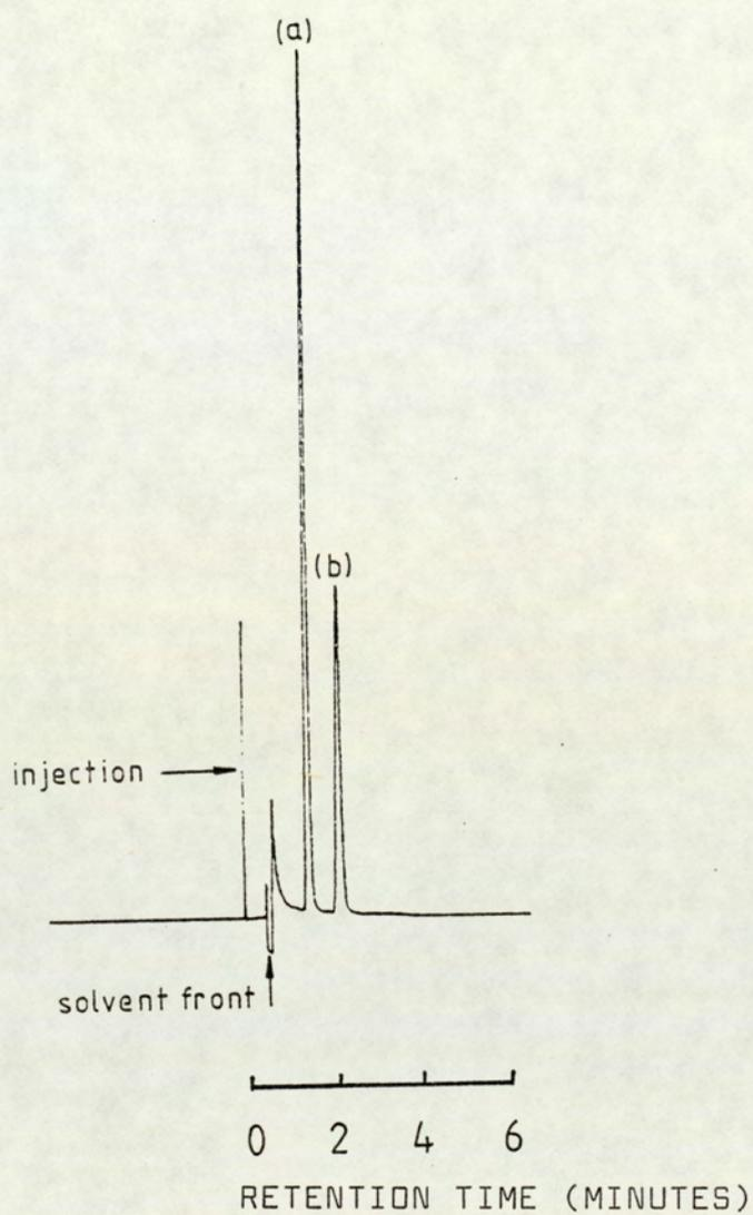
Fig. 31 Gas chromatogram of a standard solution containing 30 $\mu$ g/ml TMU (a) and NEF (b) in acetone.
