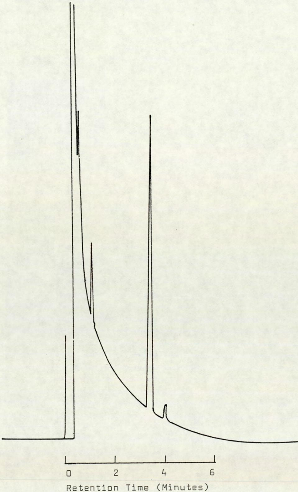
Fig. 11B Gas chromatogram of liver microsomal extract containing 50um HEM. The sample was prepared according to section (3.2.1). Peaks (a) and (b) correspond to retention times of HMM and PMM respectively.
