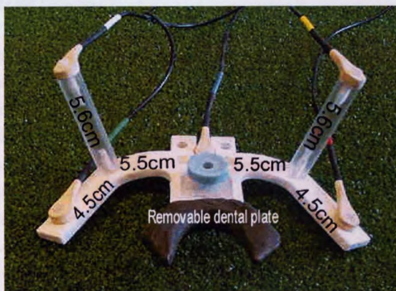
Figure 2-4. The bite-bar with the coils attached. The measurements indicate the distances between the coil locations on the same plane. The PAL and PAR coils are on the extreme arms of the device while the NA coil is located half way between. Two additional coils are raised by 5.6 cm with respect to the other coils. The removable dental plate carries the subject's dental impression.
