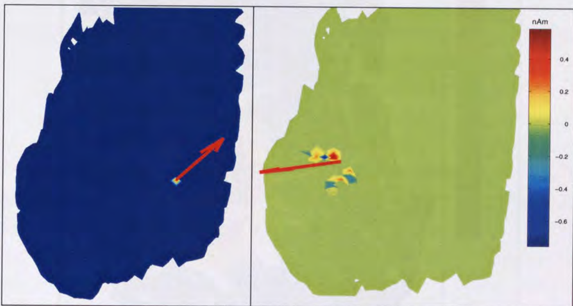
figure 4-17: Examples of impulse responses typically found with FOCUSS when the identity matrix is used as initial weighting matrix. The source spaces are viewed from the right-back. The left panel shows an ideal impulse response. The one element with a value of 1 is at the location of the original source (indicated with the red arrow). Note that no colourbar is given for this figure; dark blue represents a value of zero. The right panel shows an impulse response for which the maximum value is not in the same location as the original source. Additionally, there are non-zero elements surrounding the original source. Note however that the vast majority of elements in the impulse response have a value of zero.
