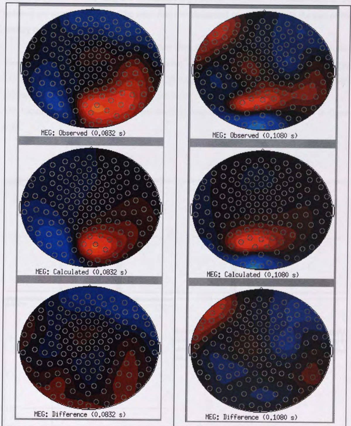
figure 6-19: Recorded magnetic field, magnetic field induced by the (unconstrained) two-dipole model and the difference between the recorded and calculated magnetic fields. Left panel: field maps at 83ms. Right panel: field maps at 108ms. Note that the difference maps did not contain a distinct dipolar pattern (compare with figure 6-17).
