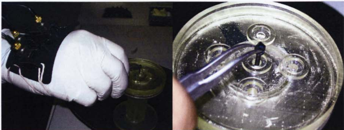
Figure 5.5: Accelerometer Placement and demonstration of micro-manipulation task of holding within a 4 mm hold a 2mm pin grasped between tweezers. The surgeons were asked to remain standing during this operation.
