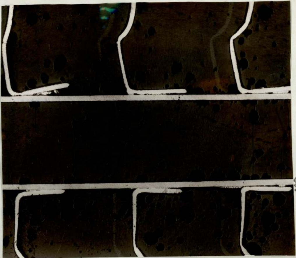
8) Unit B30 3J. Close up of a poor fin to tube bond. (x22). Fin Solder Tube
