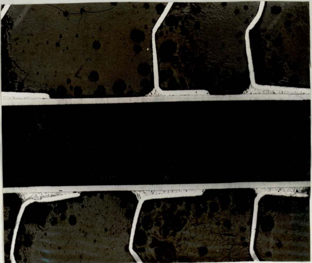
9) Unit B30 3E, close up of a good fin to tube bond - note the width of solder layer. (x22).
