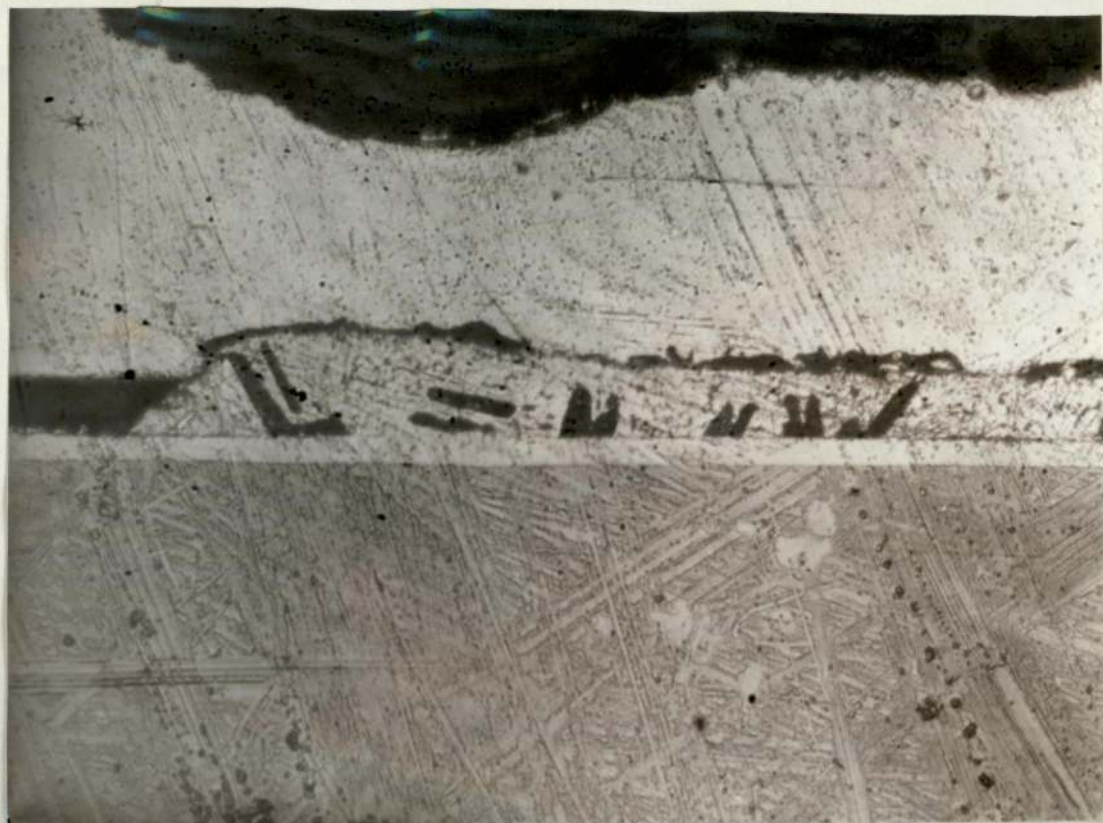
10) Close up of a corroded joint - corrosion along the interface of the fin and the solder (x400). corrosion
