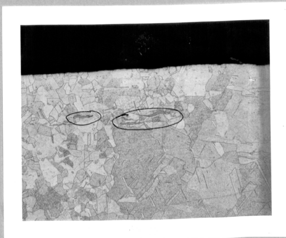
X150. Skin pipe shown (circled) in metal grain of copper tube.
