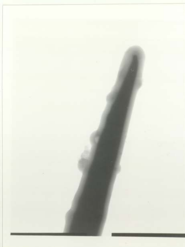
Fig. 3.14 Electron micrographs of (a) tungsten tip free from contamination (b) after been contaminated with hydrocarbon .
