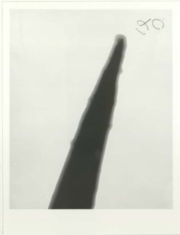
Fig. 3.12 Transmission electron micrographs of tungsten tip (a) before coating (b) after coating with a 0.06 \mu\text{m} layer of resin. (Magnification = 30240X).
