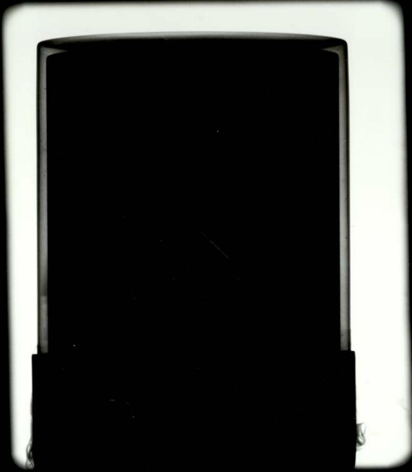
Figure [5.1] X-ray photograph of NaI(Tl) (7.62 cm x 7.62 cm) crystal, showing the location of the crystal inside the package
