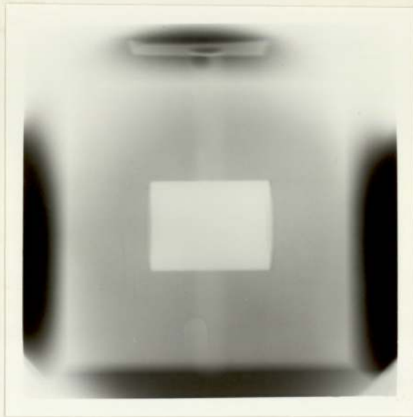
Figure (3.8) Radiograph of perspex phantom obtained with K X-rays of Mo for 50\mu\text{A} proton current and 15 minutes.
