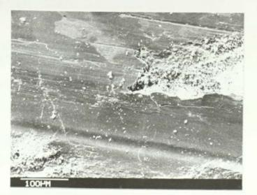
FIGURE 3.52 Typical Oxide Edges from EN8 Experiments.
