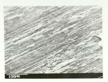
FIGURE 3.42 Topography of Worn Pin from EN8 Experiment at 100°C (4.9N).
