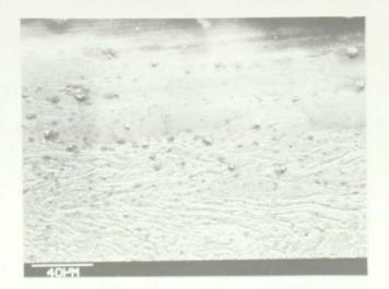
FIGURE 3.57 Tapered Microsection through EN8 Room Temperature Pin (34.3N).
