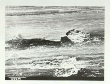
FIGURE 3.50 Topography of Worn Pin Surface from 68.7N Load EN31 Experiment at 300°C.
