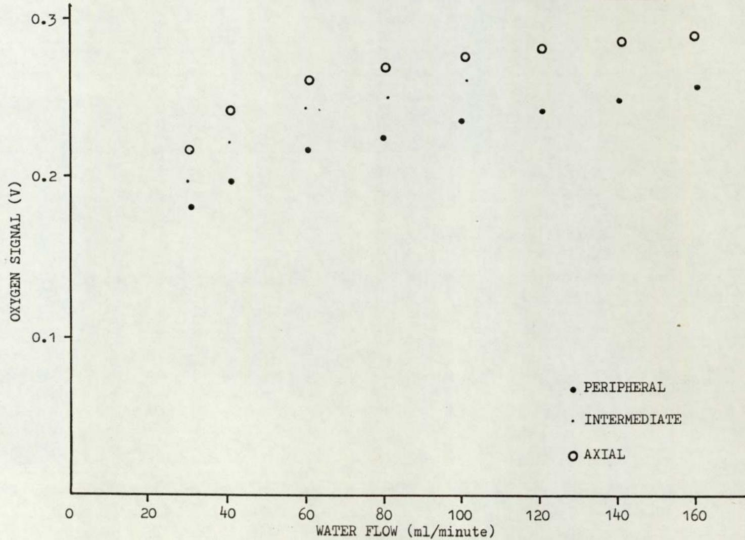
FIGURE 48 : Effect of catheter position on  $N_2$  flow dependence
