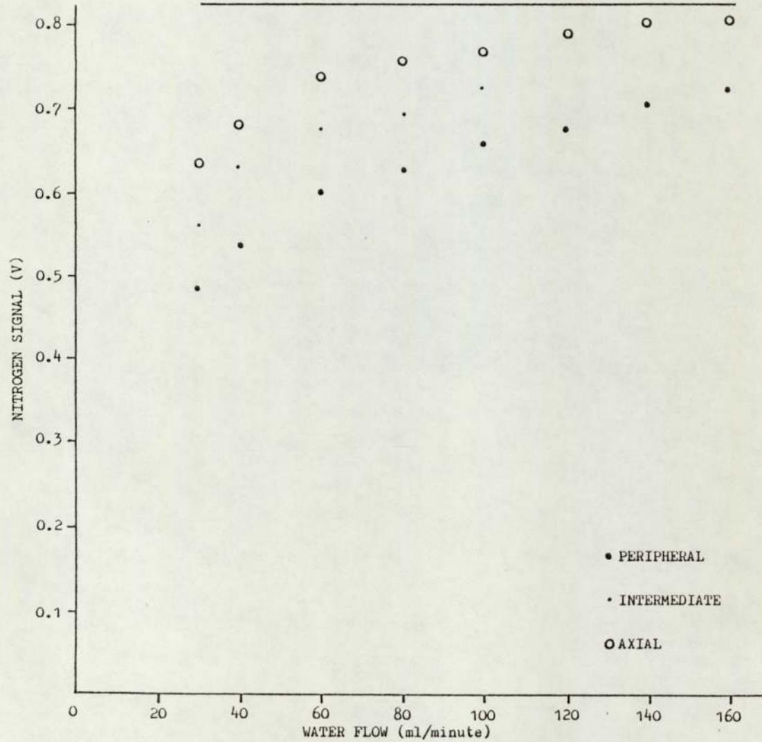
The catheter was positioned along the axis of a 9 mm diameter tube. The nitrogen signal was recorded as a function of water flow rate, firstly using the peristaltic pump to propel the water, and secondly letting the water flow through under gravity. Results are given in Table 30. Figure 49 shows that in the second case, for which the water flow was more likely to be laminar, the signals were generally lower than in the first case, in which the flow was pulsatile.
