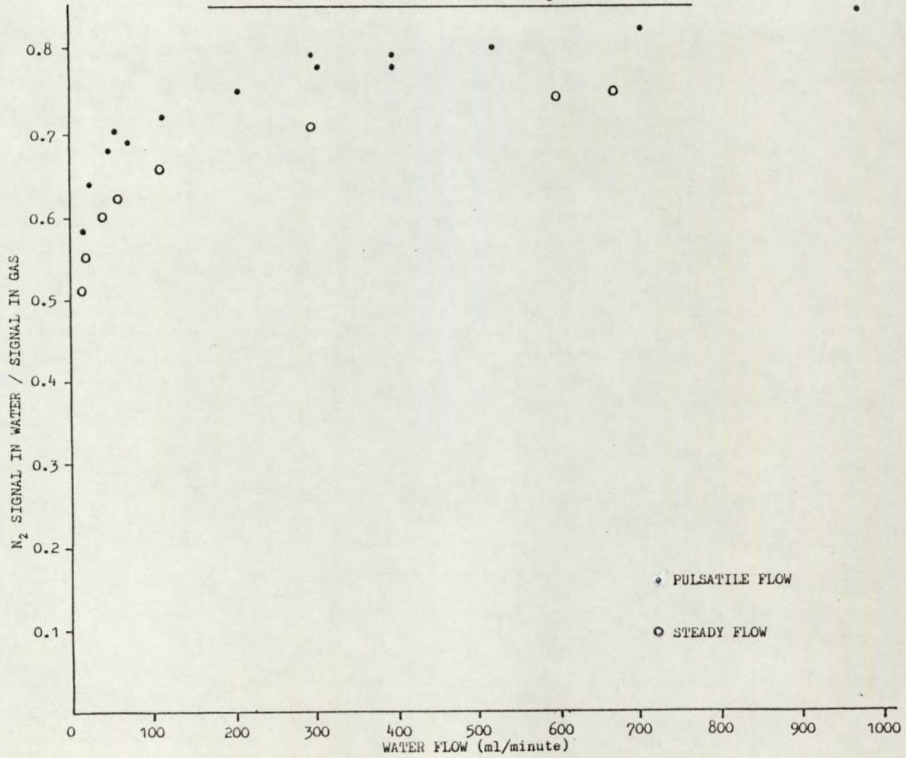
The catheter was positioned axially, then peripherally and finally in an intermediate position along a 9 mm diameter tube. The mass spectrometer nitrogen signal was recorded as a function of flow rate at each of the 3 positions, the water flowing in each case under gravity rather than by pumping. The results are given in Table 31. Figure 50 shows how the flow dependence is shifted according to the catheter's position.
