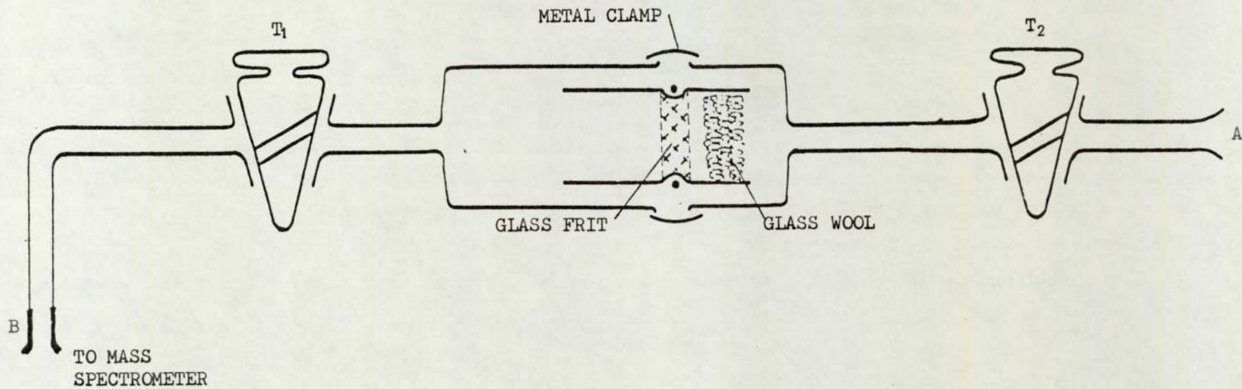
FIGURE 52 : First inlet system for content measurements
