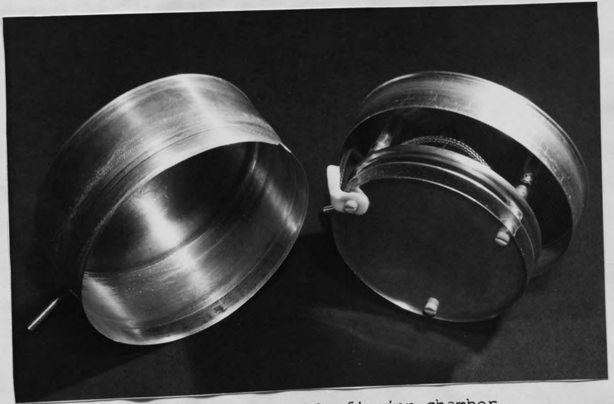
Fig. 8.3 The back-to-back double fission chamber
