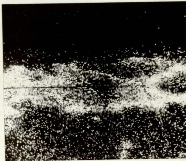
Figure 3.5 a) Electron-probe X-ray distribution image of Fe showing nodular character of oxide. b) Secondary electron image of (a). (Magnification x 190.)
