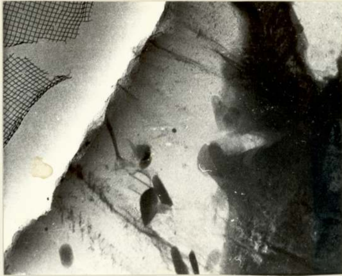
Figure 4.28 Microradiograph of a rock (Schist) sample, obtained by copper radiation at an electron accelerating voltage of 20 KV and a target current of 6.5 \mu A. Overall magnification 50x.
