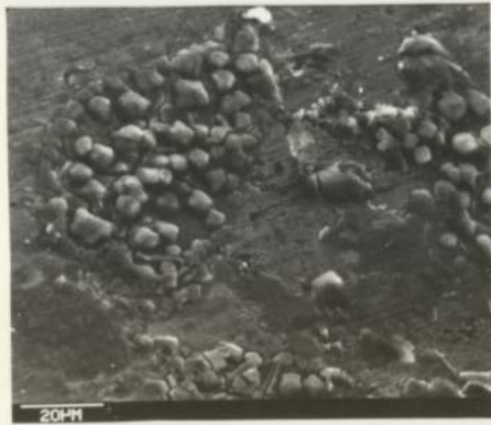
b. Cracking and spalling to form wear particles
