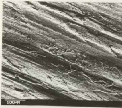
a. Wear from 24.5 to 196 N - 4\text{ms}^{-1}
