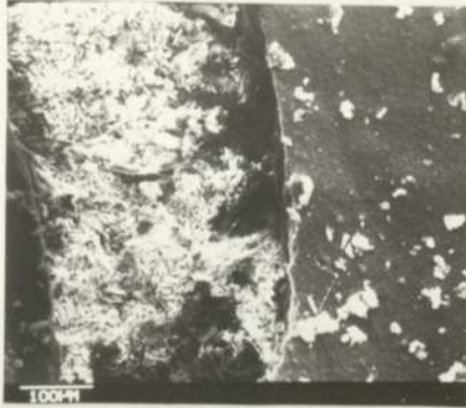
a. Wear debris mixed with graphite 122.6 N \cdot 4ms -1
