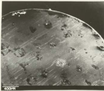
a. Resemblance to pitting failure 245\text{ N} - 1\text{ ms}^{-1}
