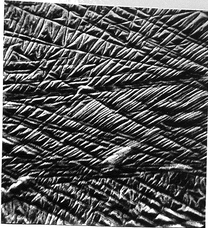
APPEARENCE OF CORRUGATIONS IN FILM COOLED OVER 400 MINUTES X 3.6K
