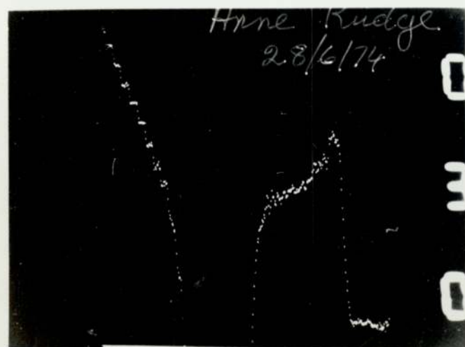
Fig. 6.6 A trace of an in-vivo ulna of a dialysis patient, 26 years old, on a low protein diet
