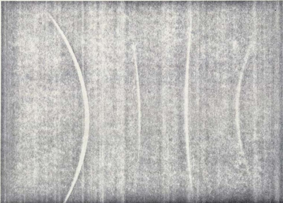
Fig. 94.3. Glancing-angle, edge-irradiated X-ray diffraction pattern from a surface worn under extreme pressure conditions with dibenzyl disulphide (d.b.d.s.) as the additive
