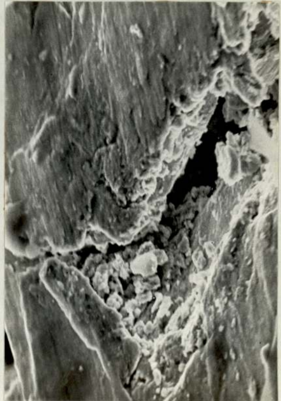
FIGURE 3.42 S.E.M MICROGRAPHS OF BRONZE WEAR SURFACES TAKEN FROM DRY WEAR TESTS.
