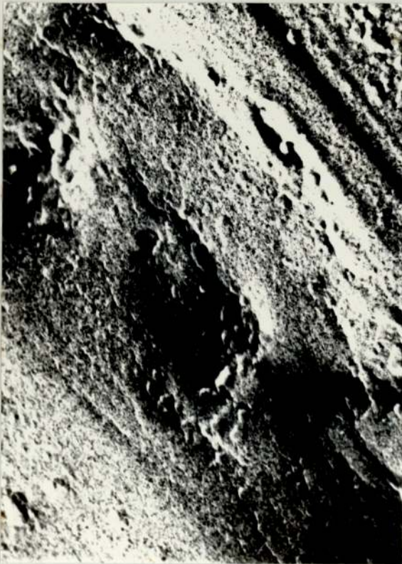
FIGURE 3.44. CARBON REPLICA OF A BRONZE WEAR TRACK ON STEEL FROM KEROSENE PLUS HITEC TESTS. ( \times 6400 ).
