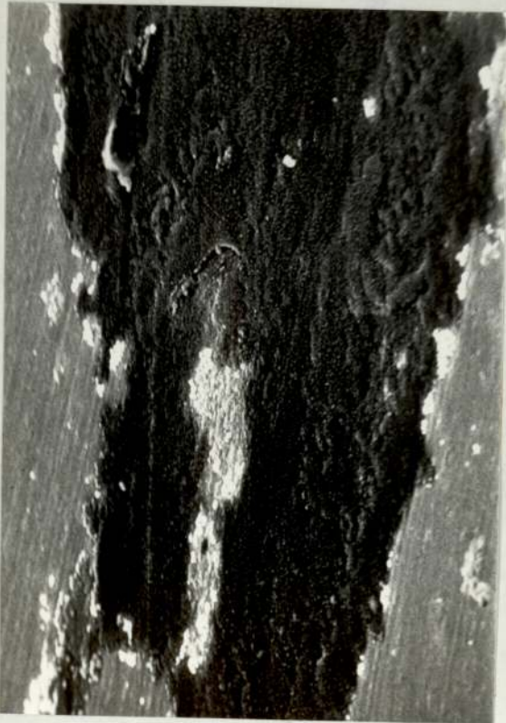
FIGURE 3.37 S.E.M MICROGRAPHS OF ALUMINIUM BRONZE WEAR SURFACE FROM KEROSENE PLUS HITEC TESTS.
