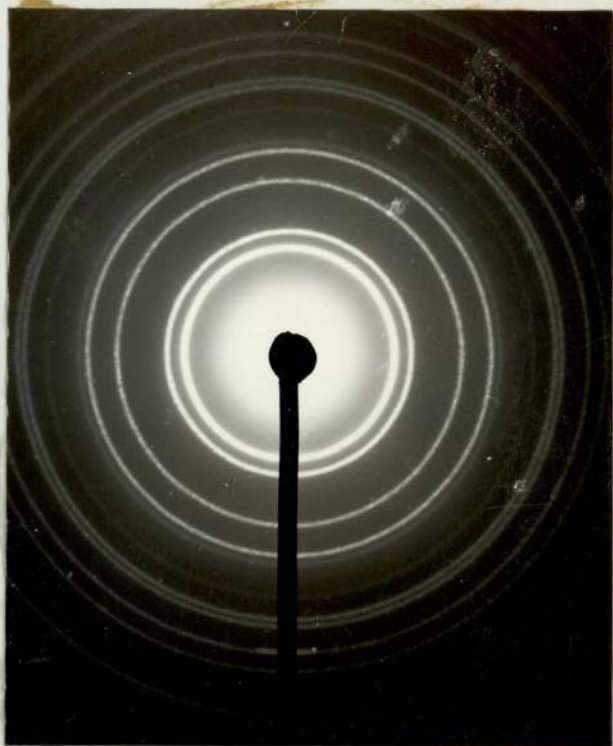
DIFFRACTION PATTERN OF PURE ALUMINIUM.
