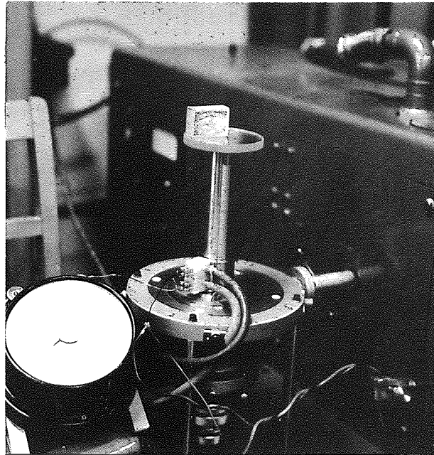
Fig. 3.4.3 The miniature rotation-free projector lens mounted on the optical bench of the 'Intercol' electron microscope.
