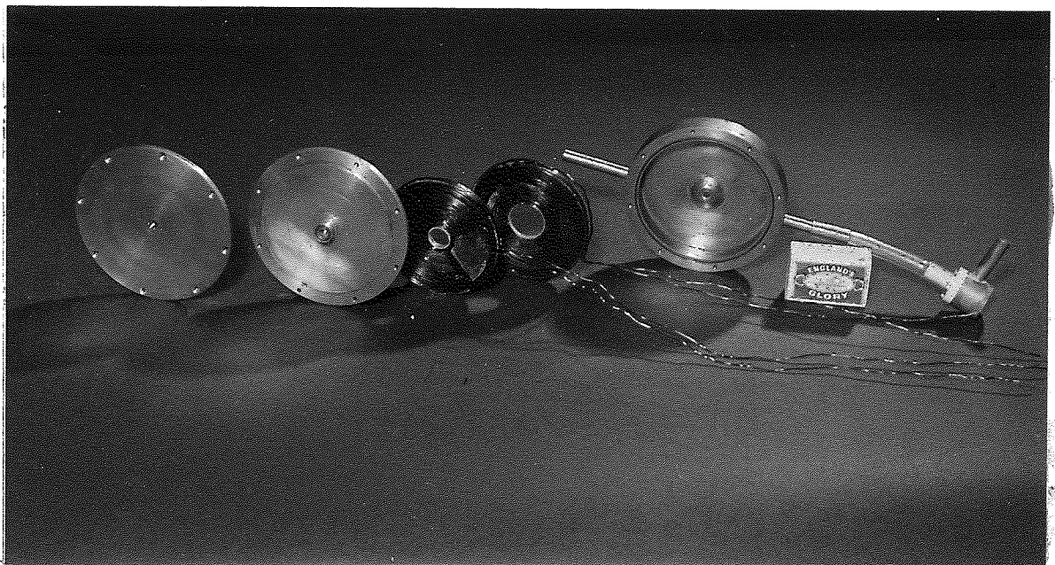
Fig. 7.1.2 Components of the experimental miniature objective lens with its interchangeable brass and iron lids.
