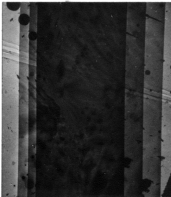
Fig. 8.3.3 Superimposed "zoom" rotation-free images of molybdenum trioxide crystal.
