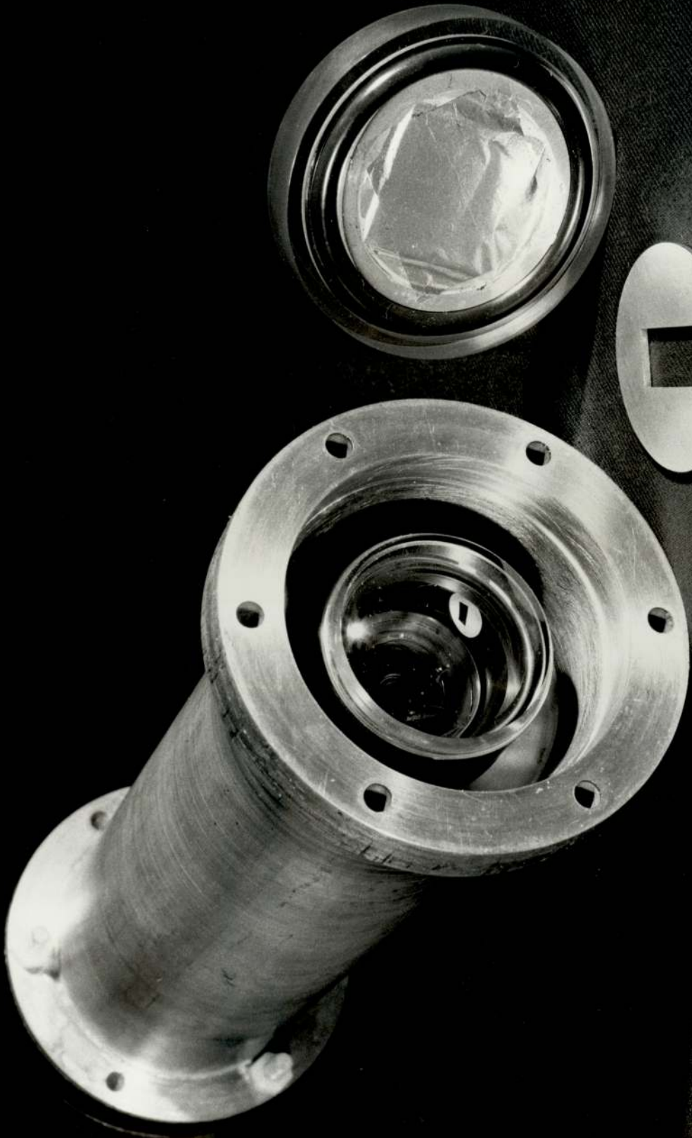
Figure 4.5 The alpha-detector photomultiplier, light pipe flange and aperture plate.
