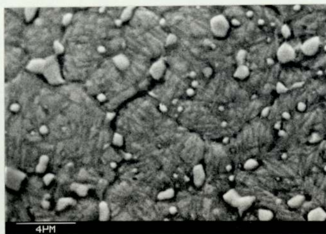
Fig.104: Scanning electron micrograph of AISI M2 high speed steel, showing a microstructure consisting of carbides in a martensitic matrix. 2% Nital etch.
