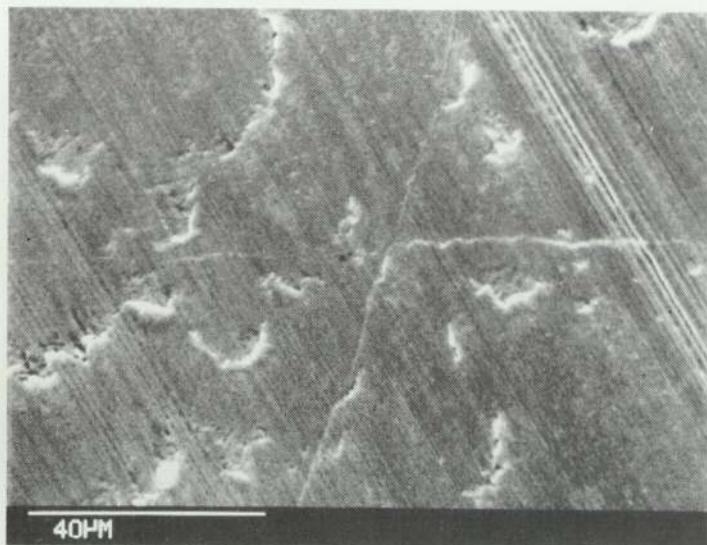
Fig 11. Scanning electronmicrograph of worn area of untreated hard chromium, showing microcrack.
