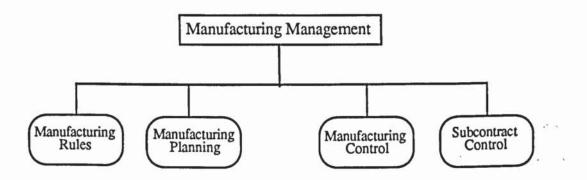
Figure 5.1 The Four Major Functions of the Manufacturing Management System
