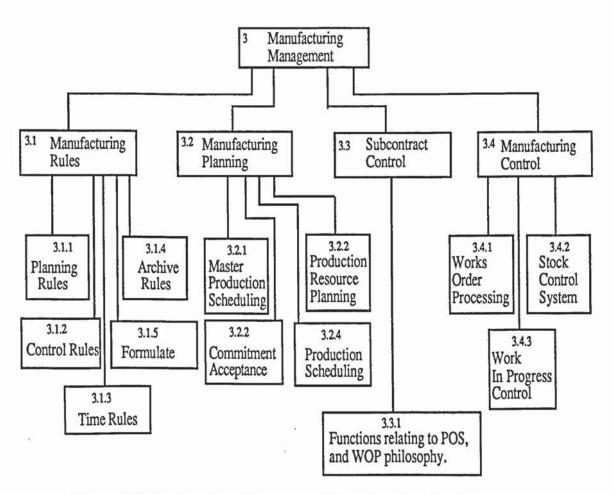
Figure 4.9 The Functional Structure of the Manufacturing Management.
