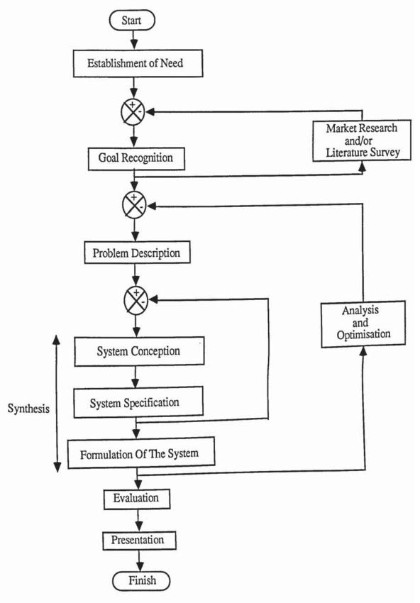
Figure 4.1 The Stages of The Design Process
