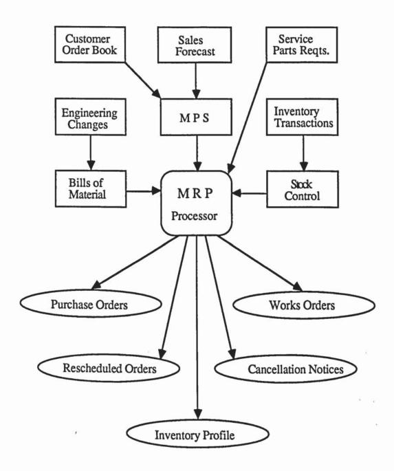
Figure 7.1 Structure of a Material Requirement Planning (MRP) system
