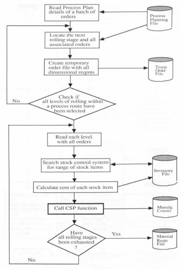
Figure 10.3 The Functionality of the CAMO System and the Integration of the CSP Module.
