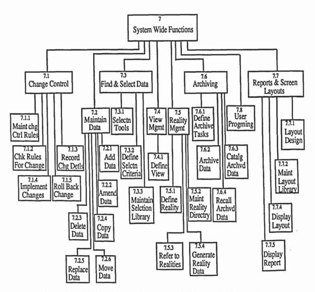
Figure 4.13 The Functional Structure of the System Wide Function.
