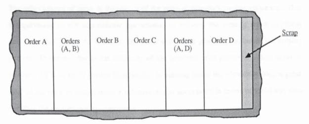
Figure 10.1b An Example of One-Dimensional Cutting Pattern With Material Scrap.
