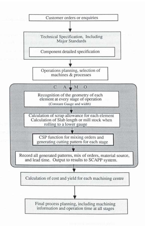
Figure 7.9 The information flow chart from customer orders to final process plans.
