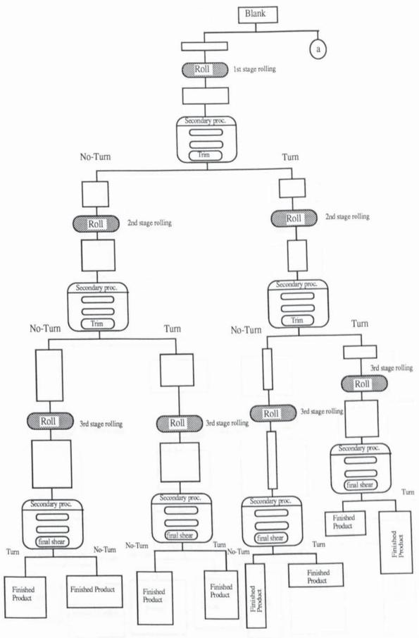
Figure 7.6 (a) The Process Rlanning Route Generated by SCAPP.
