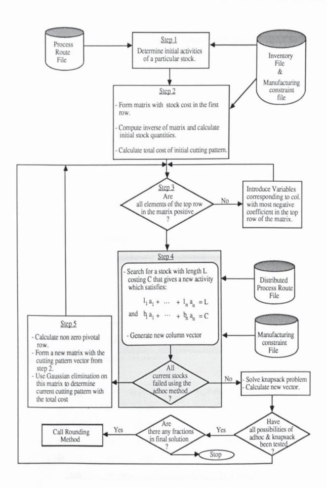
Figure 10.4 The One-Dimensional CSP Software Logic.
