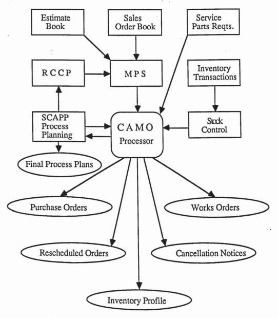
Figure 7.4 The structure of Computer Aided Material Optimisation (CAMO) system
