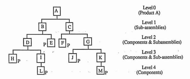
Figure 7.2 The Structure of the Bill Of Material (BOM)
