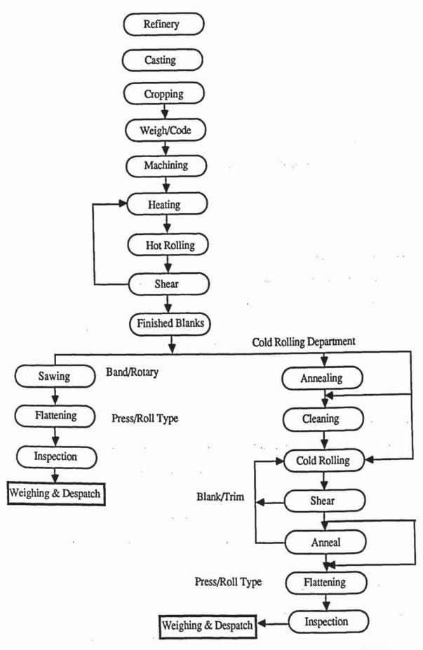
Figure 3.2 An Example of The Process Flow Chart in the Rolling Mill Industry.
