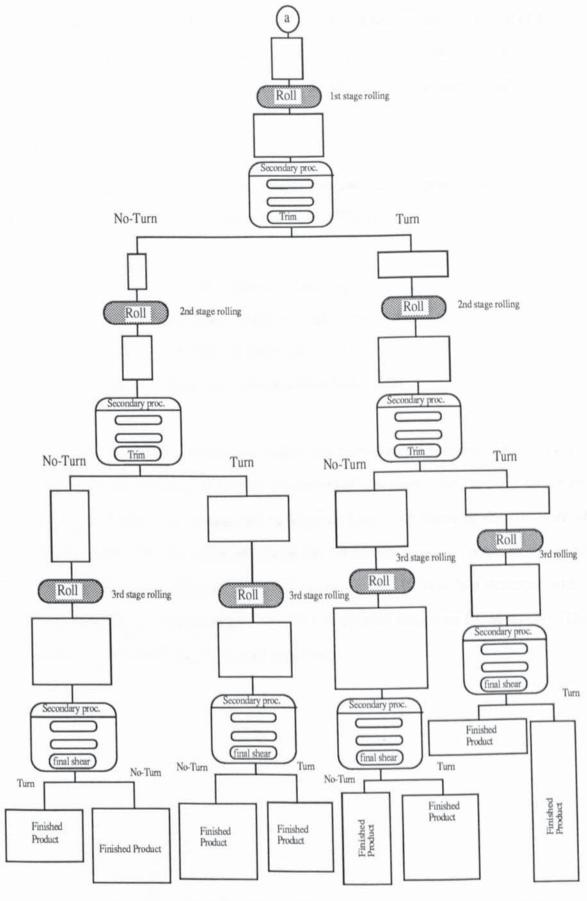
Figure 7.6 (b) The Process Planning Route Generated by SCAPP.
