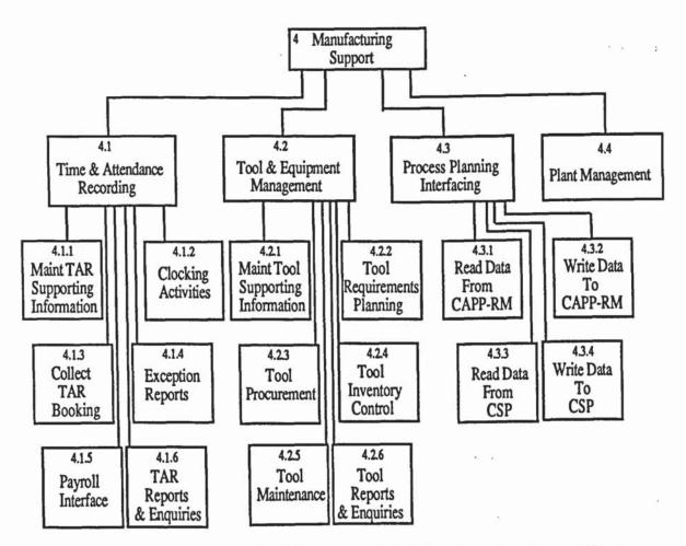
Figure 4.10 The Functional Structure of the Manufacturing Support System.
