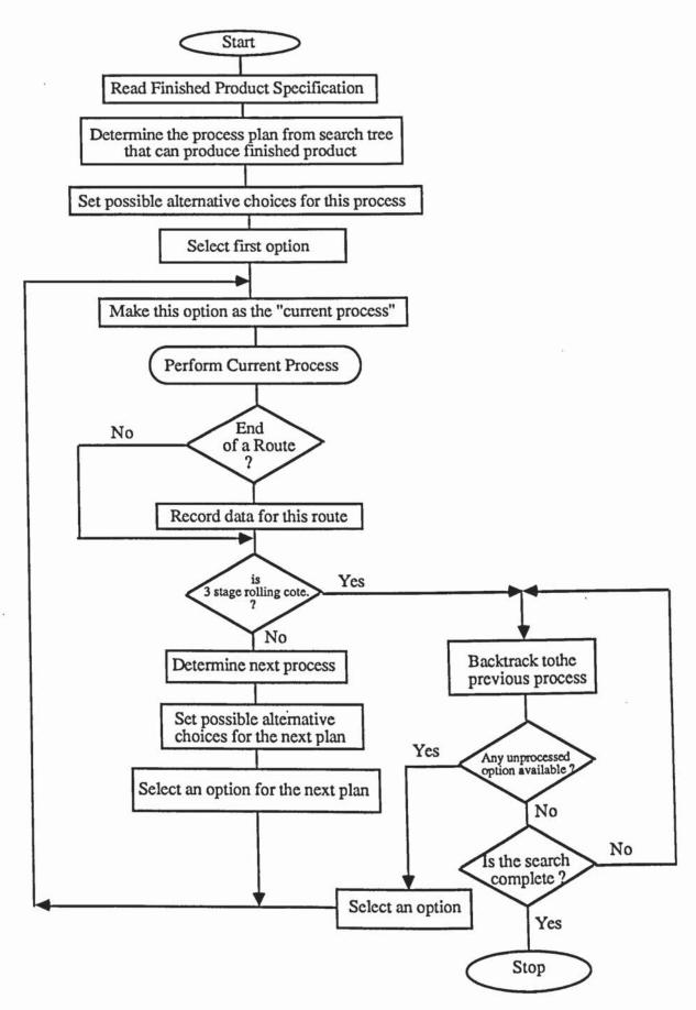
Figure 7.5 The Process Planning Logic Used by SCAPP.
