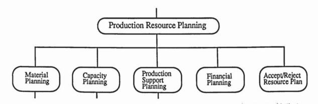
Figure 5.8 The Production Resource Planning Module and its Functions.
