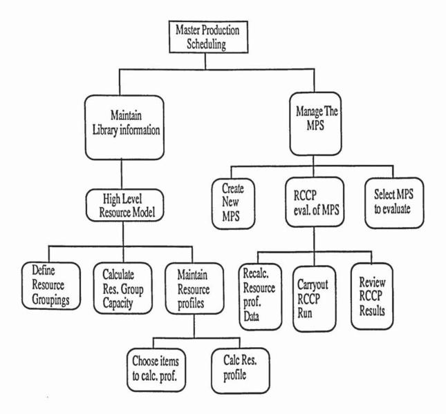
Figure C.1 The Functions of The MPS Module.
