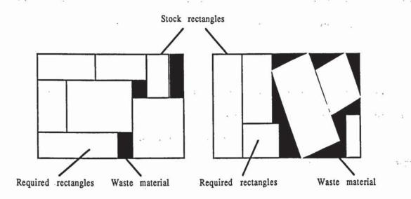
Example of an orthogonal cutting pattern Example of a non-orthogonal cutting pattern
