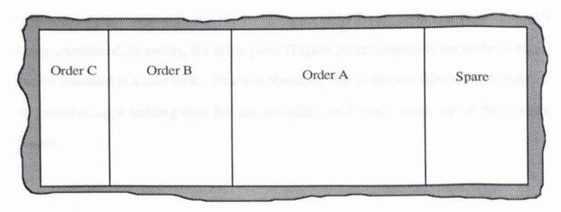
Figure 10.1c An Example of One-Dimensional Cutting Pattern With Material Spare.
