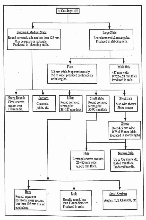
Figure 2.2 The Production Chart of Rolled Products, their Uses and Sizes.
