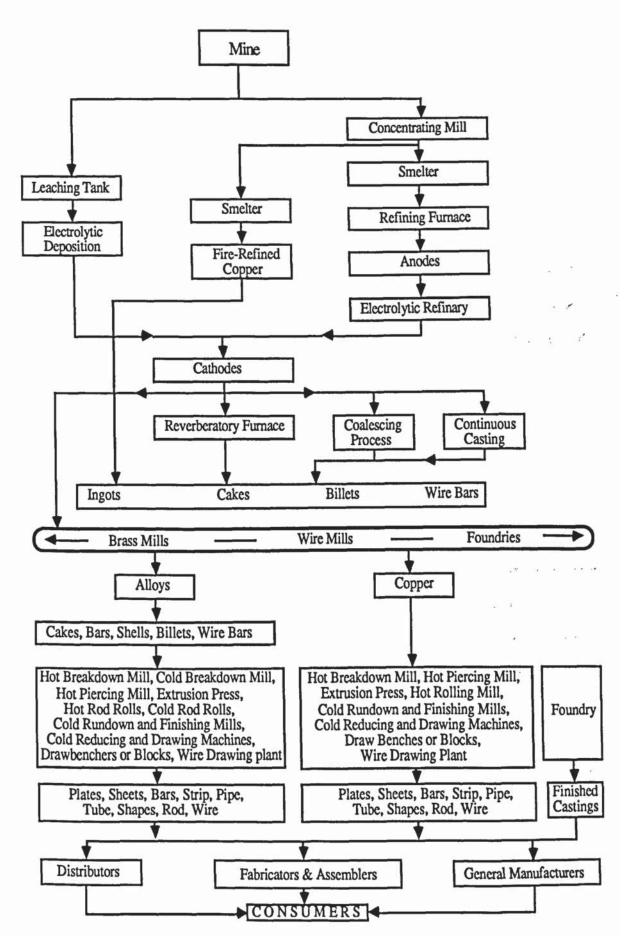
Figure 2.1 The Manufacturing Stages of Rolled Products From Mining to Consumers.
