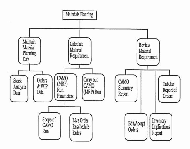
Figure C.2 The Material Requirements Planning Functions.
