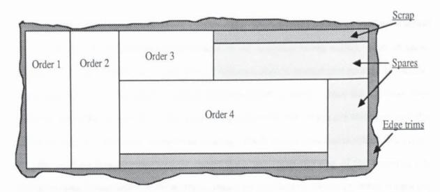
Figure 10.1a An Example of a Two-Dimensional Cutting Pattern With Three Types of Material Losses.
