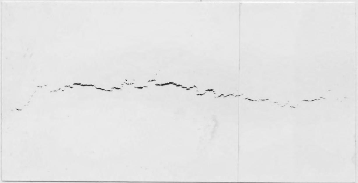
Figure 104. Hydrogen induced 'stepwise' crack found in steel 5.
