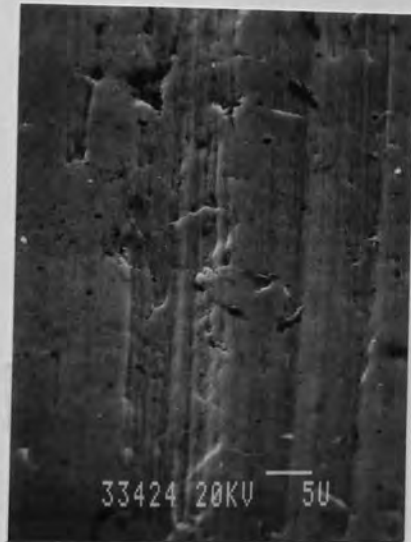
(c) Wear scar of as-deposited surface
