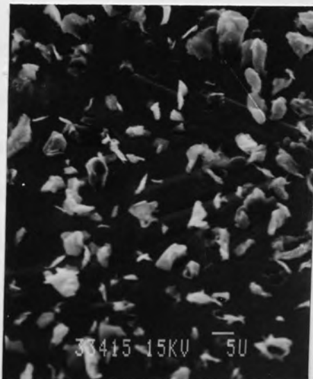
Figure 44. The adsorption of graphite flakes onto the surface during the first 30 seconds of plating from an electroless nickel-graphite solution.
