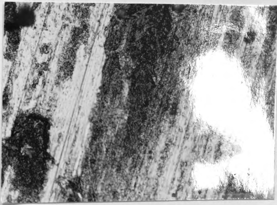
Figure 63. Optical photograph of the wear track on En 31 disc after running against a heat treated electroless nickel coated pin, sliding speed 50 cm/s, load 2 Kg
