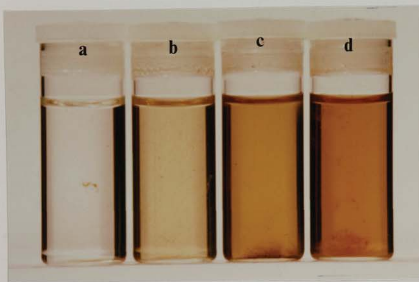
Plate 7. Change in appearance of a nominally 15 volume per cent solution of the representative PVP (Parquench 90) with increased throughput in the accelerated ageing test. (a) Fresh, (b) 10kg/litre, (c) 50kg/litre and (d) 100kg/litre.
