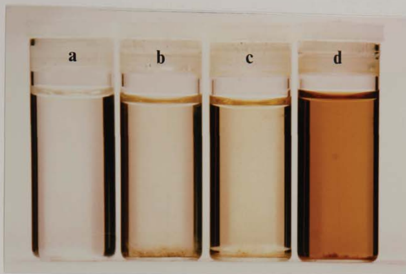
Plate 6. Change in appearance of a nominally 15 volume per cent solution of the representative PAG (Quendila PA) with increased throughput in the accelerated ageing test. (a) Fresh, (b) 10kg/litre, (c) 50kg/litre and (d) 100kg/litre.
