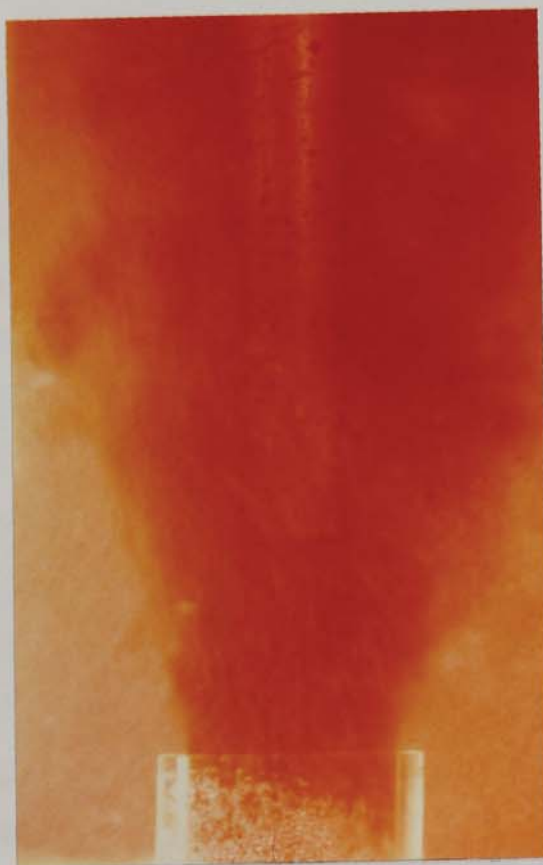
Plate 5. Flow visualization for a 15 per cent Quendila PA (PAG) solution at the standardized test conditions (probe 25mm above 25mm diameter outlet through which the 30 °C solution is being pumped at a fluid velocity of 0.5m/s).
