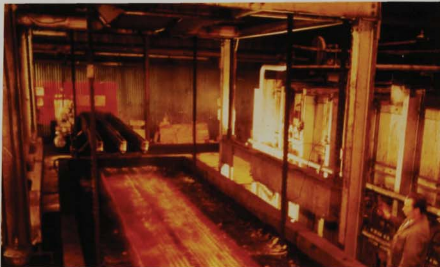
Plate 2. Quenching into a 20 per cent PAG solution following conversion to a polymer quenchant. (84)
