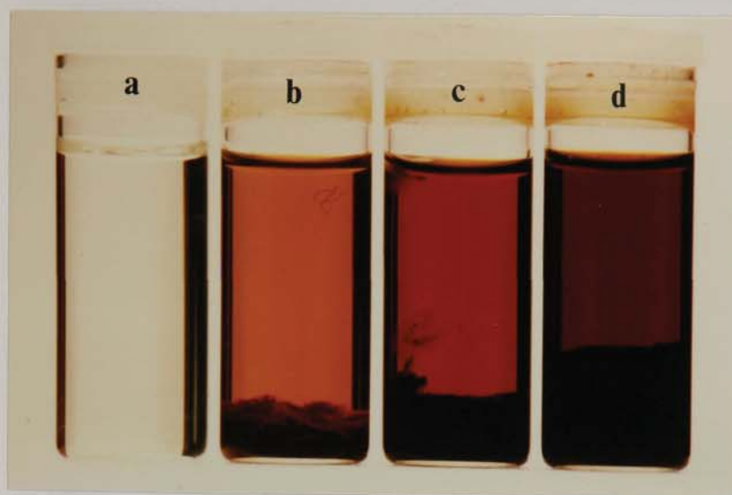
Plate 8. Change in appearance of a nominally 15 volume per cent solution of the representative Polyacrylate (Aquaquench ACR) with increased throughput in the accelerated ageing test. (a) Fresh, (b) 10kg/litre, (c) 50kg/litre and (d) 100kg/litre.
