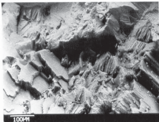
Figure 4.10 Creep fractures for alloy SRR 99 tested at 750°C
