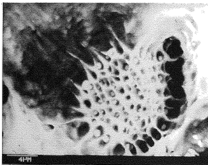
PLATE 16 : Cluster of inclusions (MnS) which have acted collectively to form a single void . Smaller voids exist around the individual inclusions themselves . Steel F rolled at 1100^{\circ}\text{C} . Hounsfield tensile specimen .
