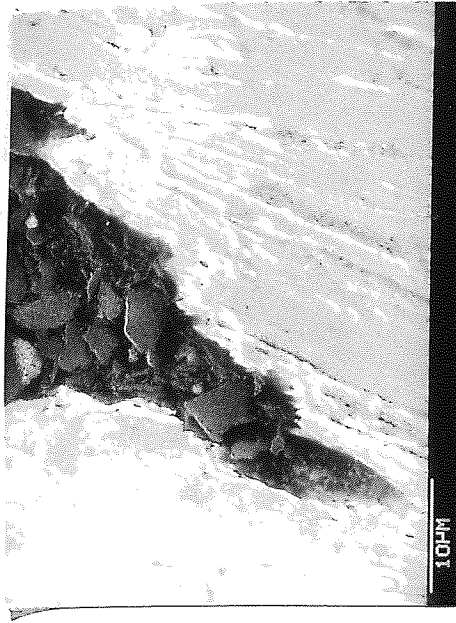
PLATE 82 : Example of cross section through fracture surface showing cusps formed from pearlite colonies .
