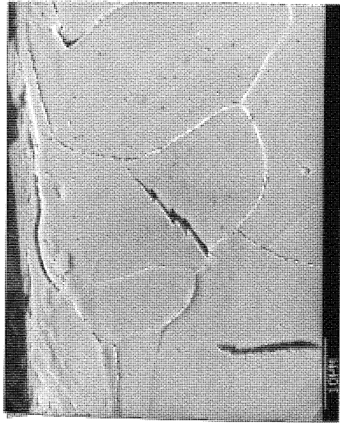
PLATE 74 : Heavily deformed region adjacent to fracture surface giving way to undeformed matrix containing transgranular cracks . Note partial decohesion of Al_2O_3 inclusion at bottom of Plate .
