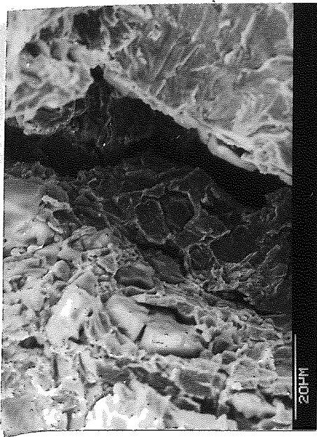
PLATE 64 : Detail of Plate 62 showing \text{Al}_2\text{O}_3 inclusions and Ca, Mn and S containing phases in the crack mouth .
