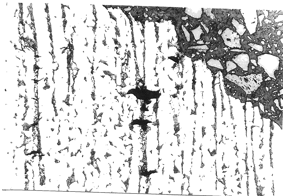
PLATE 88 : Example of cracks occurring predominantly in the pearlite bands and running perpendicular to the tensile axis . Mag.X420 .
