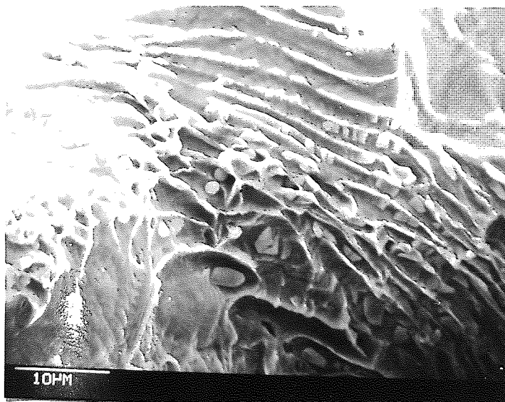
PLATE 50 : Steel F rolled at 1100^{\circ}\text{C} , longitudinal specimen, hydrogen charged . Left hand crack has arisen from large silicate inclusion (white) but is also associated with MnS networks . Whereas right hand crack has developed from a network of very closely associated MnS inclusions .
