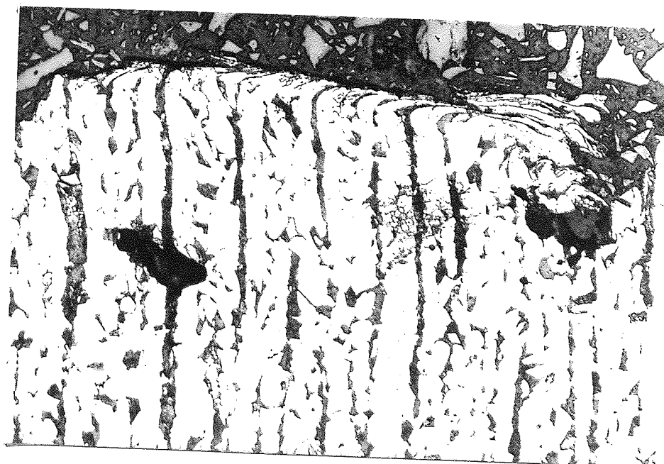
PLATE 89 : Evidence of plasticity adjacent to the fracture surface . Mag.X420 .
