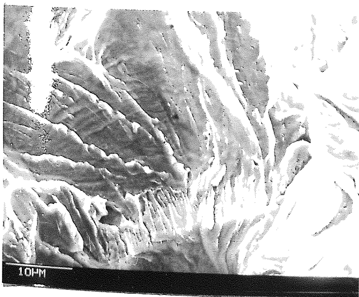
PLATE 52 : Detail of Plate 50 above, note absence of inclusions and ripples (beach marks) on the fracture surface .
