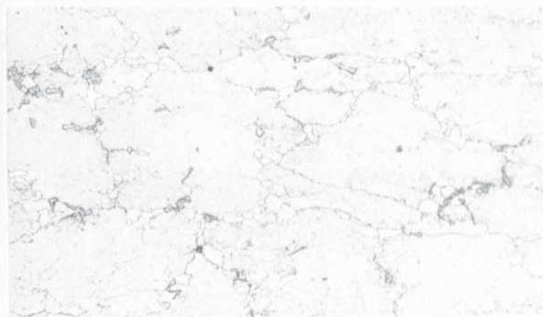
Plate 8.20: Microstructure in Transverse Section for Alloy 2014 T651, x160.
