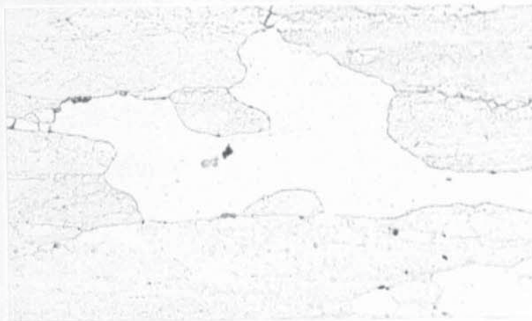
Plate 8.22: Grain Structure in Transverse Section for Alloy 7475 T736, x400.
