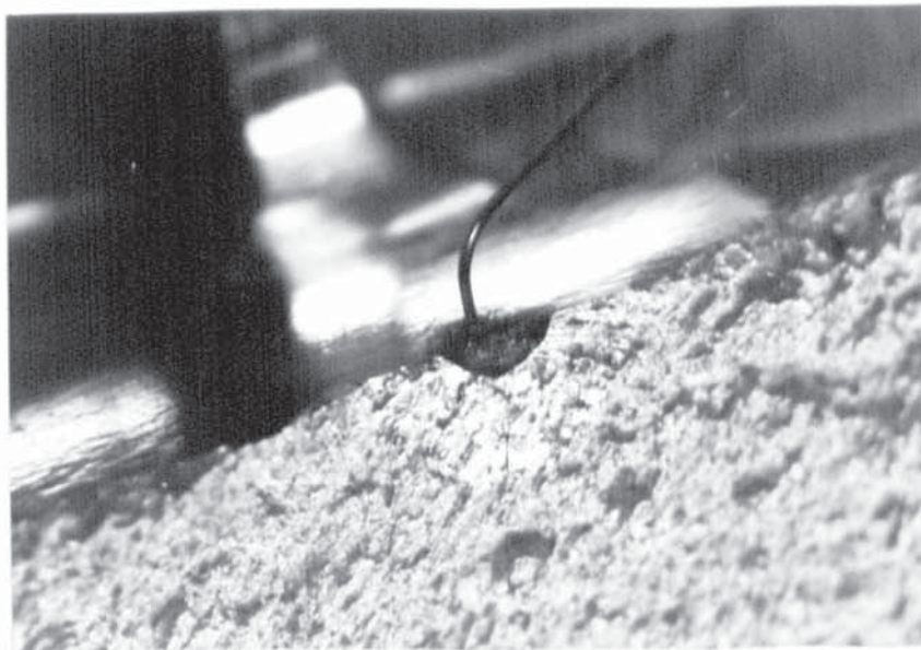
Plate 8.4 : Thumbnail Crack from Spark-Machined Notch.
