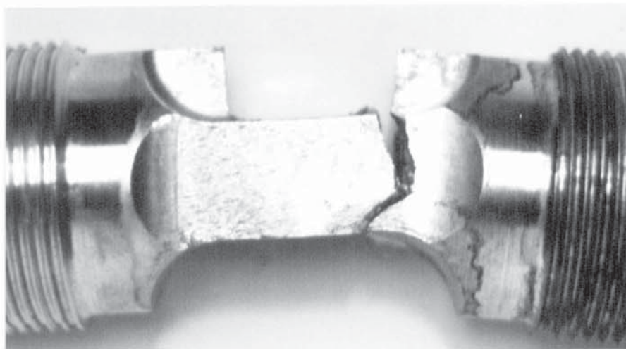
Plate 8.17 : Failure of Front-Face Crack Specimen.
