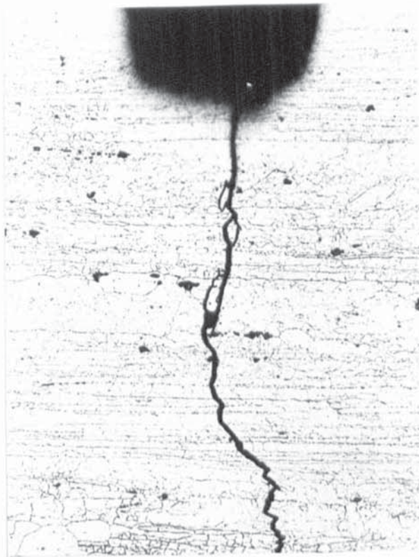
Plate 8.12 : Through-Thickness Crack Growth from a Spark-Machined Notch.
