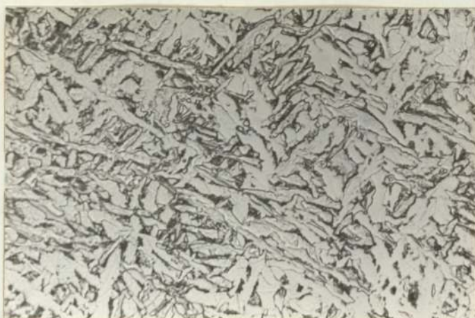
0.021 %wt Nb, Series F. Cooling Rate (CR) 4.2°C/sec.
