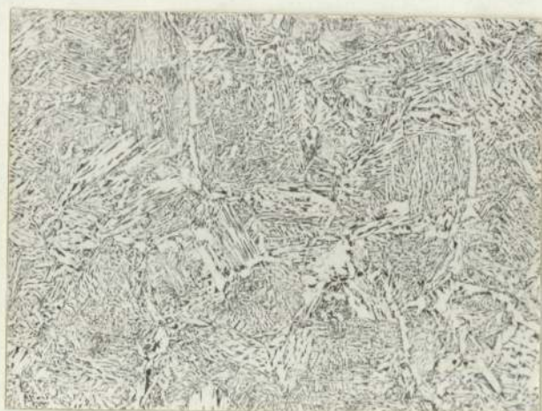
A. Specimen DD13 Cooling Rate(CR), 3.9°C/sec.
