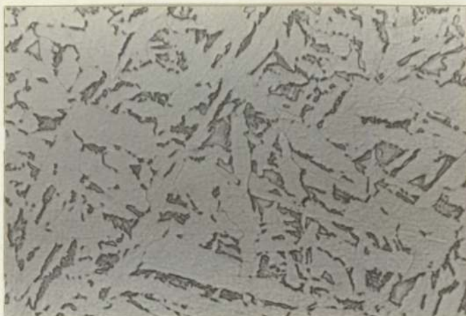
0.020 %wt Ti, Series D. Cooling Rate (CR) 6.9°C/sec.
