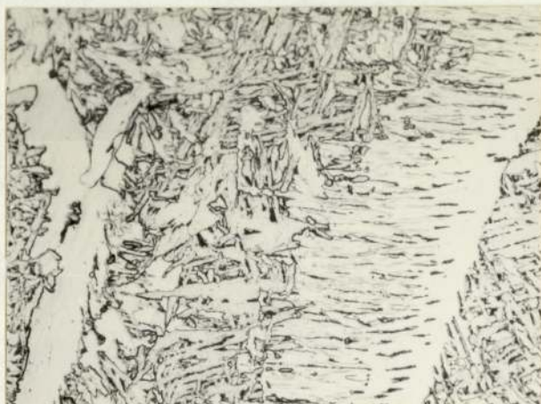
A. Specimen J1. Cooling Rate(CR), 4.0°C/sec.
