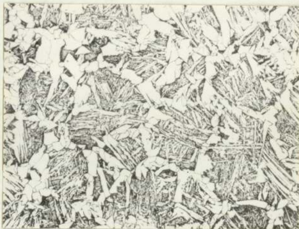
A. Specimen DA4. Cooling Rate(CR), 4.2°C/sec.
