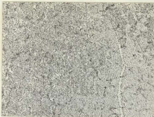
A. Specimen B8. Cooling Rate(CR), 5.5°C/sec.
