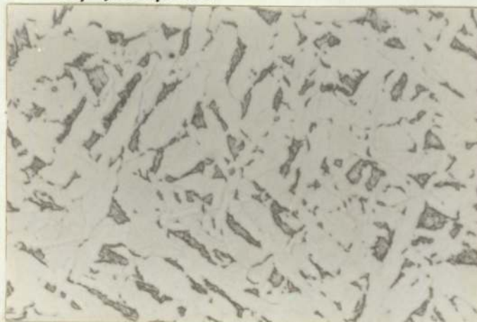
0.088 %wt V, Series C. CR, 6.1\text{ C}/\text{sec.}
