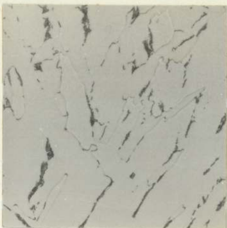
A. 0.05%wt Carbon Alloy Series J. Cooling Rate 8.0°C/sec.
