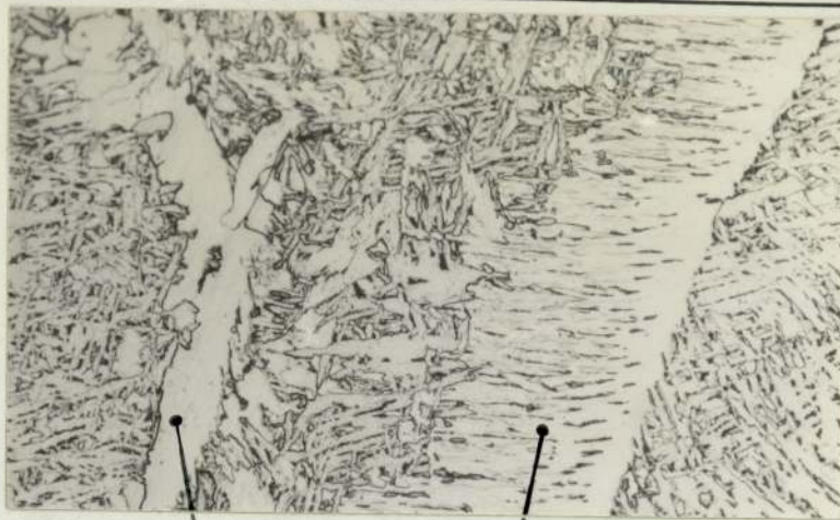
A. Primary Ferrite And Ferrite Side Plates. Mag. X160.
