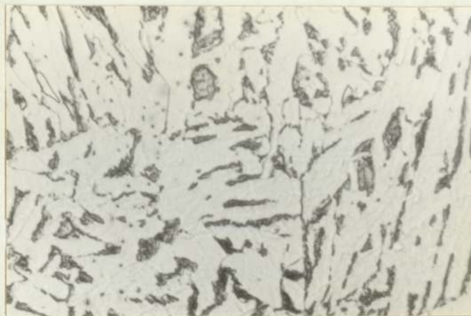
0.021 %wt Nb, Series DF. Cooling Rate (CR) 4.3 °C/sec.
