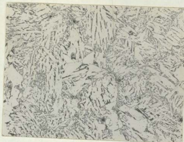
A. Real Weld Metal Produced Using A Tungsten Inert Gas Process And Welding Conditions Which Gave A Cooling Rate Of 4°C/sec. ( \Delta T_{800-500^{\circ}\text{C}} ).
