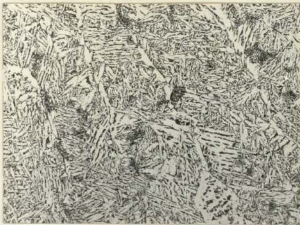
A. Specimen G4. Cooling Rate(CR), 3.9°C/sec.
