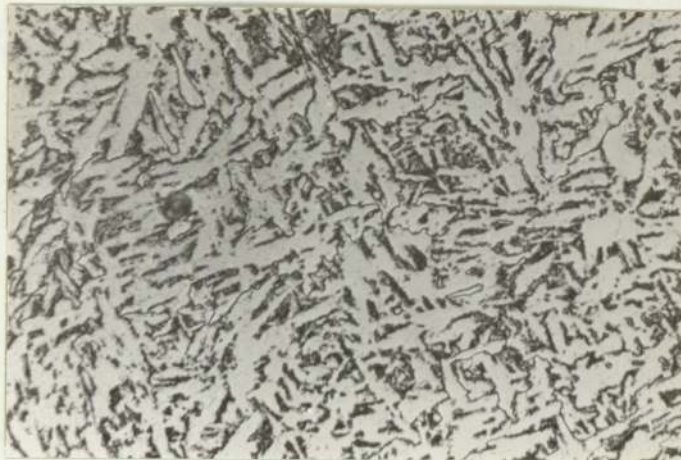
0.063 %wt Al , Series I. CR, 4.5^{\circ}\text{C}/\text{sec}.
