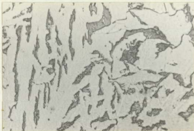
0.024 %wt Al, Series DH, Cooling Rate (CR) 4.9^{\circ}\text{C}/\text{sec} .
