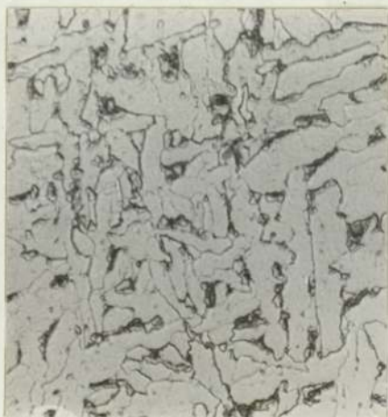
A. 0.05%wt Carbon Alloy. Cooling Rate 4°C/sec.
