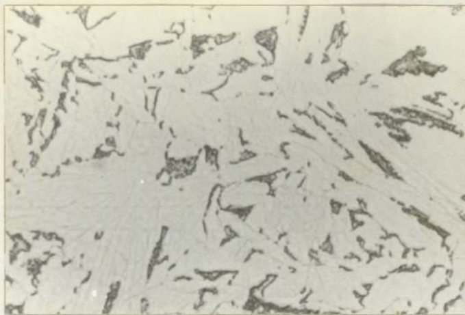
Base Alloy, Series A. Cooling Rate (CR) 7.0^{\circ}\text{C}/\text{sec.}
