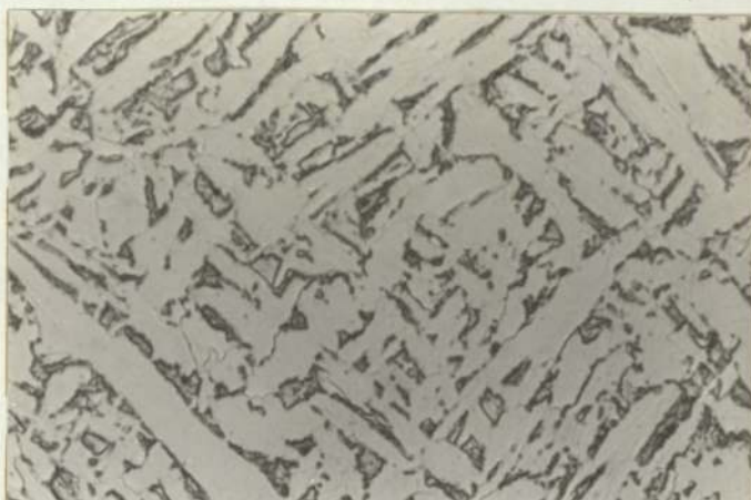
0.053 %wt Nb, Series G, CR, 7.0^{\circ}\text{C}/\text{sec}.
