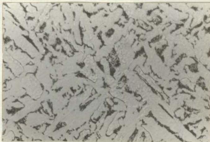
0.027 %wt V, Series B. CR, 7.2\text{ C}/\text{sec.}
