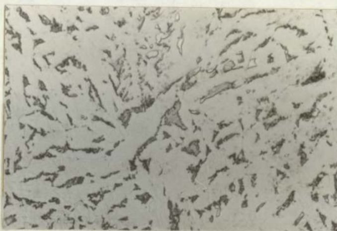
0.027 %wt V, Series DC. CR, 4.1^{\circ}\text{C}/\text{sec}.
