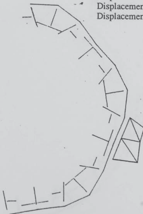
Fig. 8.24 Computed Operating Shapes for Machine B Running at 55 rpm - Group (RAD_C2_A0).
