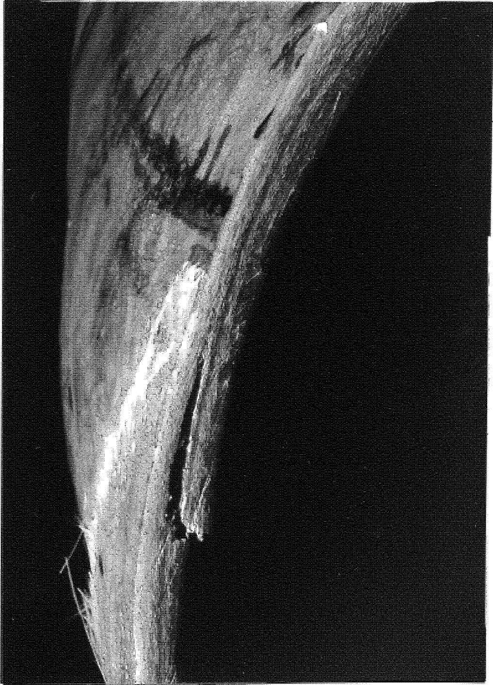
Figure (3.23c) Picture showing wall laminate splitting of bend S022.
