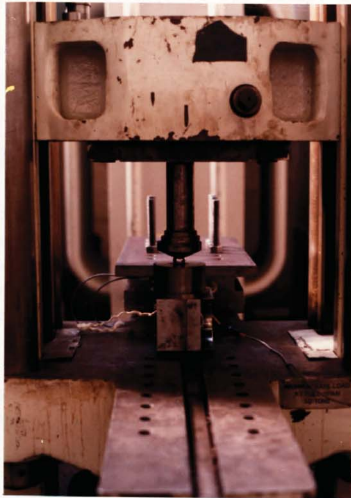
FIG 4.12 MOUNTING OF THE BENDING LOADING CALIBRATION OF A BOTTOM PINCH ROLL LOADCELL
