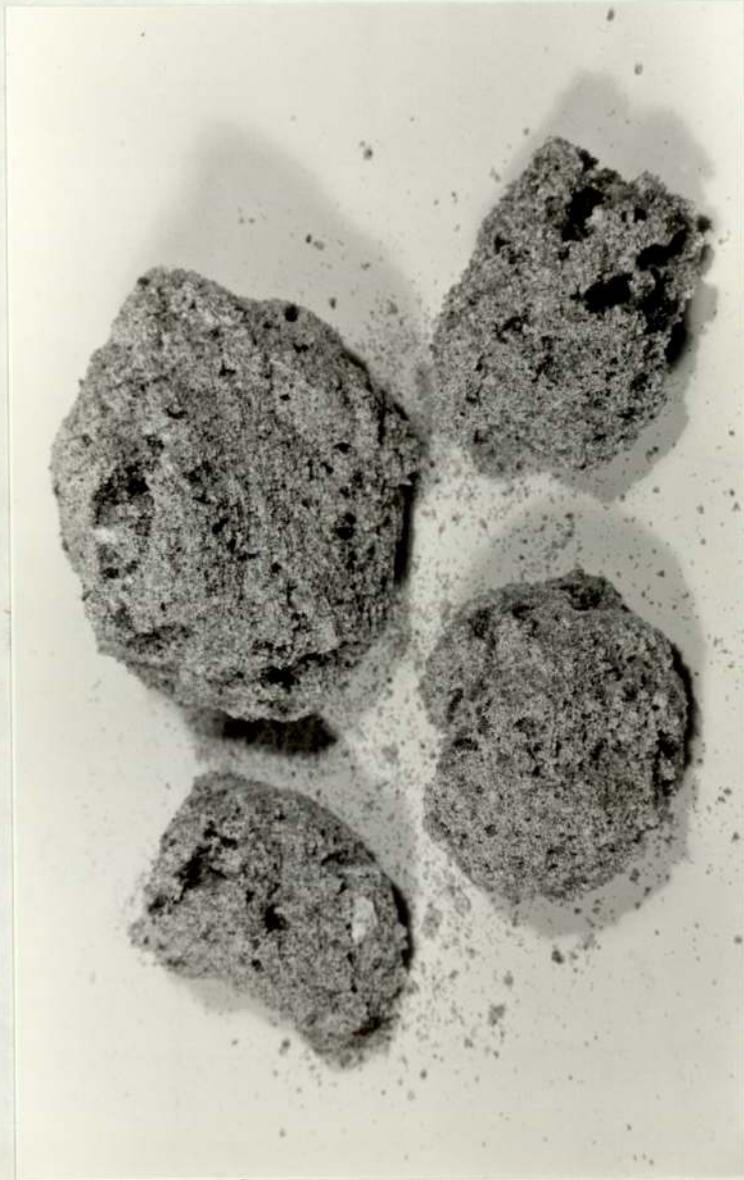
FIG. 5.22 PHOTOGRAPH SHOWING THE SINTERED BED SURFACE
