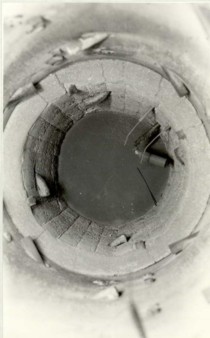
FIG. 5.23 PHOTOGRAPH SHOWING THE BURNOUT OF THE PILOT BURNER
