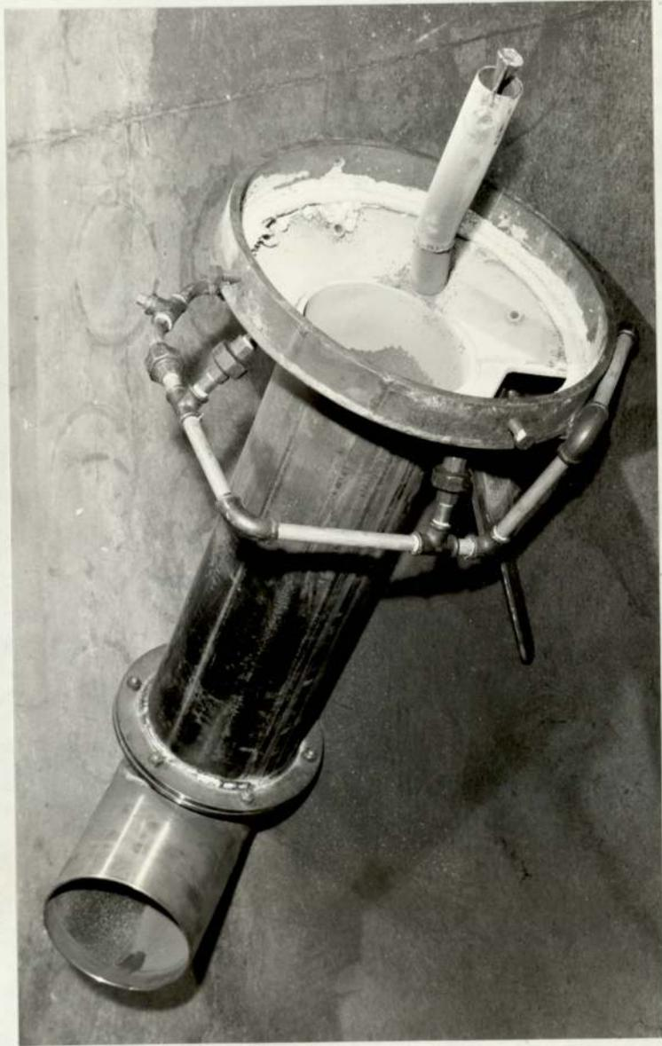
FIG. 5.2 PHOTOGRAPH SHOWING THE CONE SHAPED CHIMNEY WITH THE ATTACHED CONE FOR COAL DISTRIBUTION
