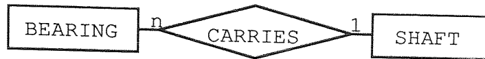
Fig 5.6 Showing a partial Entity-Relationship diagram for a database system for gearbox design
