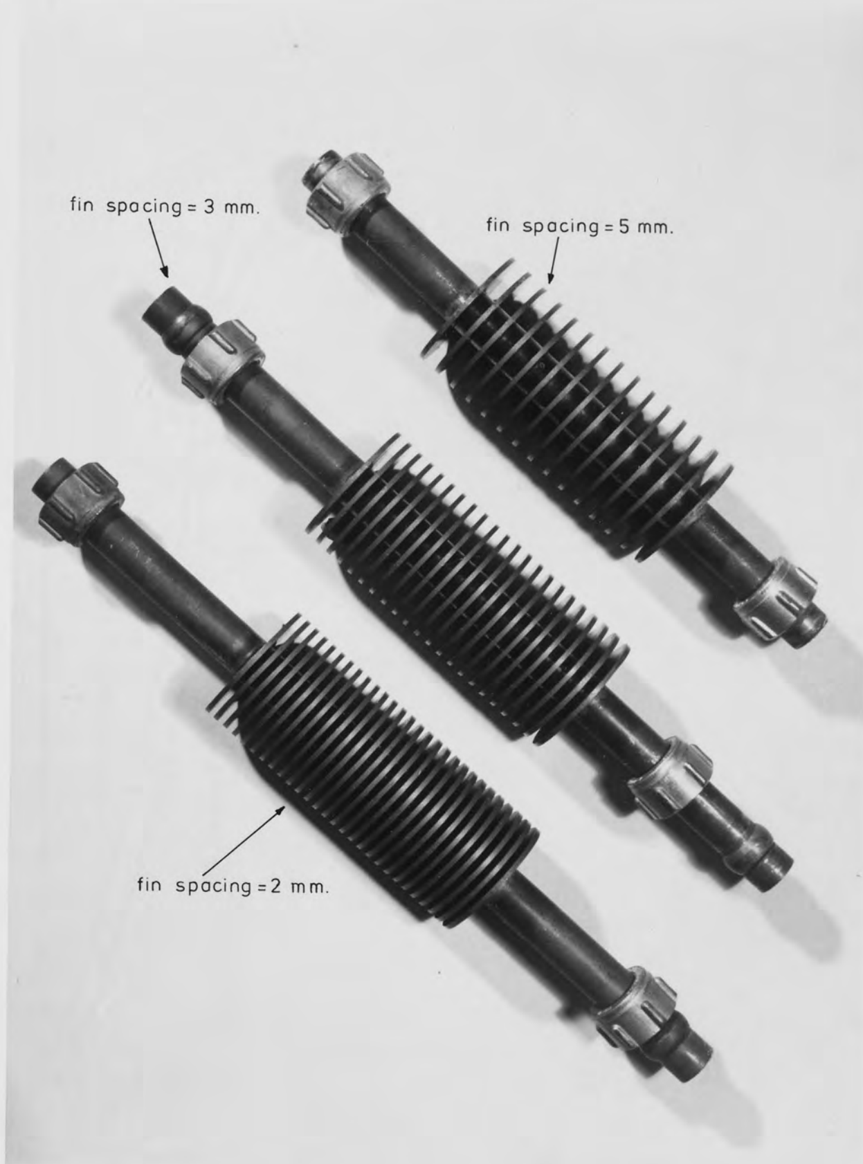
FIG.(8.2) THE FINNED TUBE ELEMENTS
