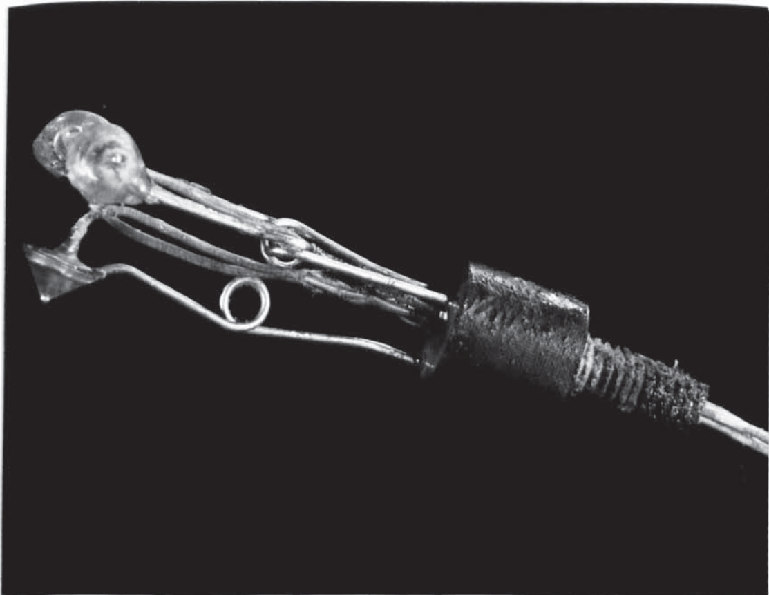
THREE POINT SLIDING CONTACT THERMOCOUPLE PROBE (Side view) P 3.9
