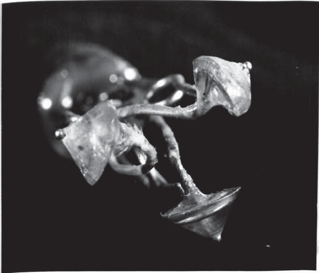
THREE POINT SLIDING CONTACT THERMOCOUPLE PROBE (End view) P 3.8
