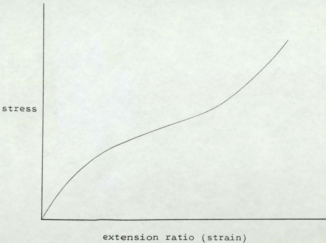
Figure 3.3: Stress-strain curve for rubber vulcanisate
