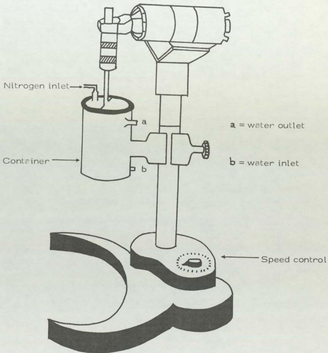
Fig. 4.1. Zigmaree Attritor used to prepare dispersion of solid antioxidants.
