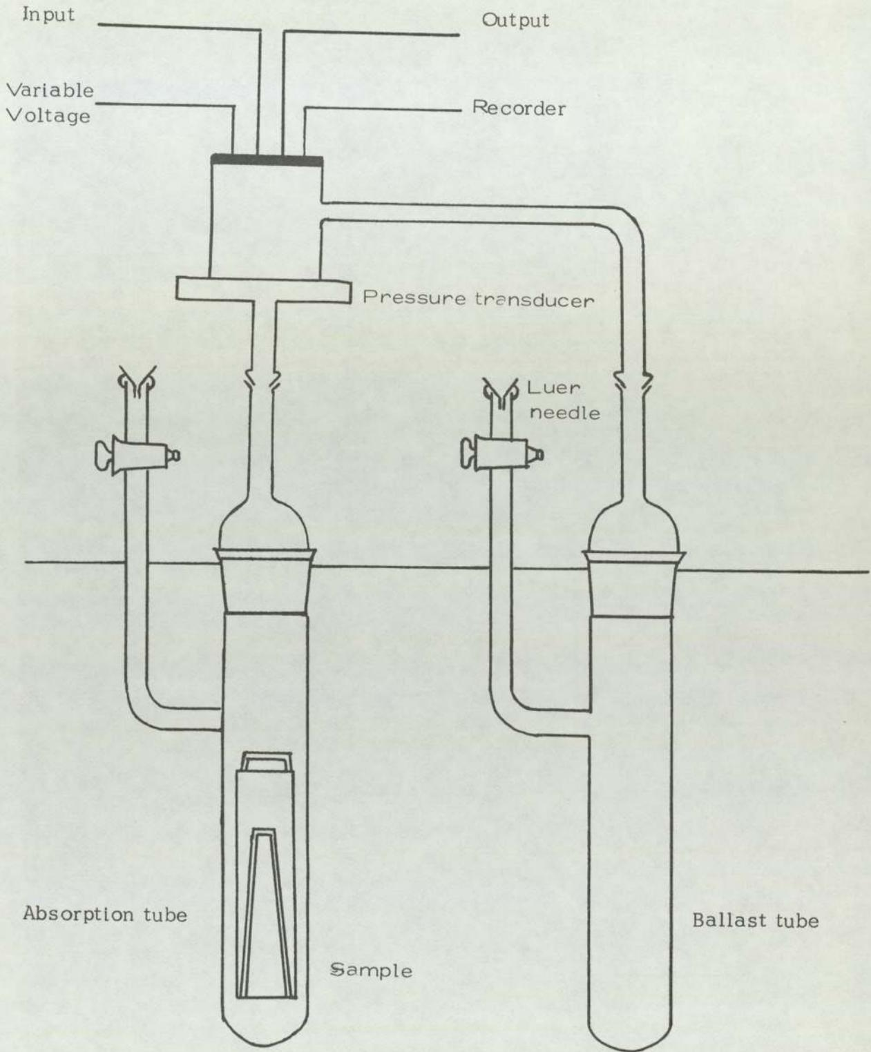
Fig. 2.9 Apparatus for oxygen absorption of vulcanisates
