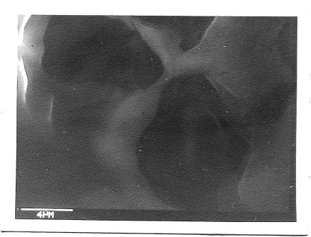
Surface of HEMA/DMAEMA/EDM terpolymer
