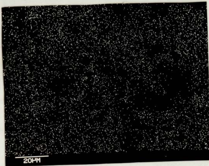
FIG. 41 SEM PHOTOGRAPH OF COPOLYMER 8 COMPOSITE CONTAINING POZZOLANIC CEMENT, PRETREATMENT AND CAESIUM CHLORIDE
