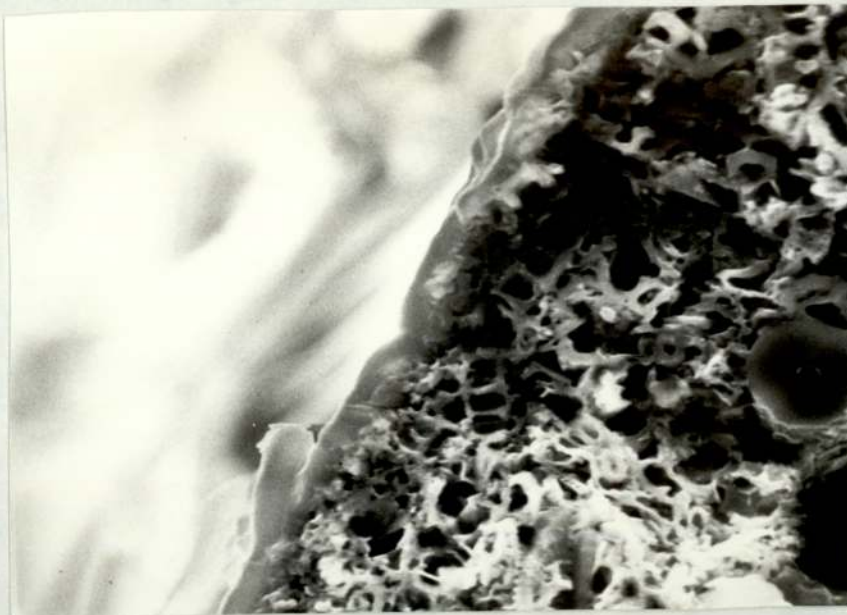
5.1 Cross-section of diatomaceous silica pellet coated with PAN.P x 1500
