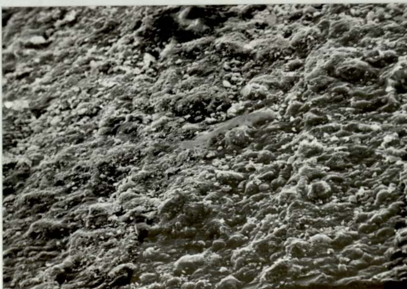
6.3 Surface of CX0136 alumina support pellet coated with PAN.P and reacted with NO at 500°C x 600
