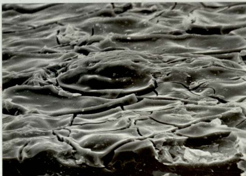
5.3 Surface of CX0136 alumina pellet coated with PAN.P x 550
